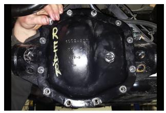
3. Place drain pan under rear differential where it can catch fluid. Remove factory plug and allow fluid to drain. Then remove bolts (x12) and differential cover.
