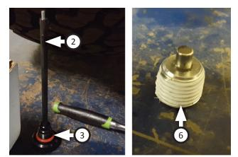
Install o-ring (3) onto dipstick (2). Wrap drain plug (6) with PTFE tape (about 2 wraps).
