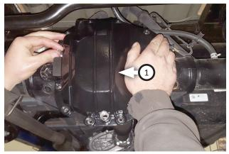
Place factory gasket (removed step 4) onto rear differential cover (1). Secure them to rear differential using screws (x2) on both sides as shown.
