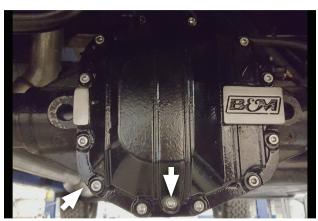
8. Install factory plug (removed step 3) and remaining screws (x10) to secure front differential cover then install drain plug.
