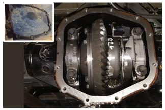
4. Remove and retain gasket from differential cover; wipe it clean and dry. Then clean mounting surface on front differential.
