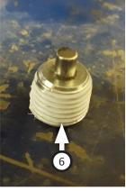
6. Install o-ring (3) onto dipstick (2). Wrap drain plug (6) with PTFE tape (about 2 wraps).
