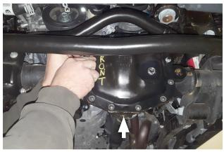
Place drain pan under front differential where it can catch fluid. Remove factory plug and allow fluid to drain. Then remove bolts (x12) and differential cover.
