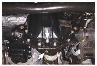
8. Install factory plug (removed step 3) and remaining screws (x10) to secure front differential cover then install drain plug.
