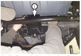
Place factory gasket (removed step 4) onto front differential cover (1). Secure them to front differential using screws (x2) on both sides as shown.
