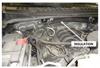
**NOTE:** On some vehicles, the firewall insulation may cover the entire firewall. The adapter can be fastened directly over the insulation, if necessary.
