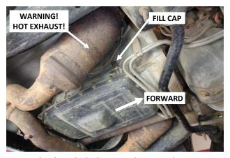
4. Under the vehicle, locate and remove the transmission fill cap. (It is located on the passenger side of the transmission, above and toward the front of the pan.) WARNING: The exhaust system is extremely hot. Wear suitable gloves and long sleeves to avoid burns.
