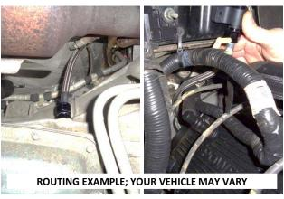
13. Route the tube (2) between the transmission and engine compartment, based on your observations in Steps 9-12.
