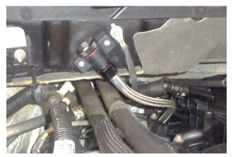
20. Wipe the dipstick and wire with a clean, lint-free rag to remove any rust preventative oil. Then install the dipstick in the tube, and tighten the knob fully hand-tight (until the o-ring is compressed).
