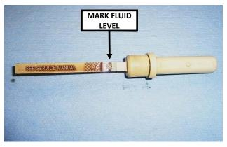
7. Mark the fluid level on the dipstick with a marker or grease pencil and carefully set it aside.
