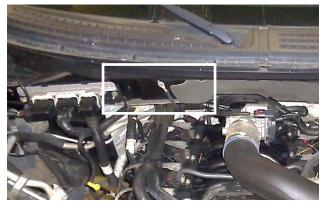
11. Find a suitable location on the passenger-side of the firewall to mount the dipstick adapter (3), while also looking for a suitable route for the dipstick tube.
