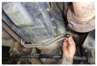
14. Remove the fill cap. If hot (expanded) fluid begins to run out of the port, reinstall the cap, start the vehicle and run it at idle, then remove the cap.
