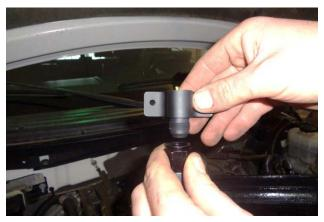
17. Thread the adapter to the top of the tube, but leave the nut loose at this time.
