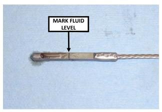
23. Remove B&M dipstick, wipe it off, and reinstall it all the way (knob fully hand tight). Then remove the dipstick again, mark the fluid level with a marker or grease pencil, and turn off the vehicle.
