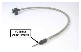
10. Also note if / when the top of the dipstick tip (where it is swaged to the cable) catches on the edge of the fitting (1).
