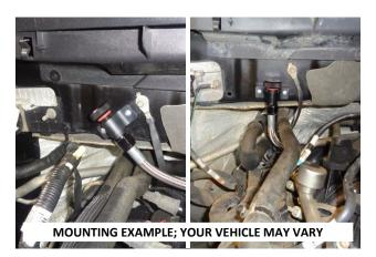
18. Use cable tie(s) to secure the dipstick tube, if required. Fasten the adapter to the chosen location on the firewall using the two self-tapping screws (4).
