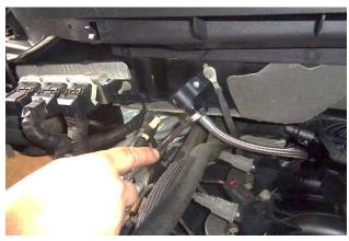
19. Tighten the upper tube nut.
