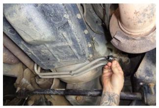
5. Blow or brush off the area around the fill cap, to prevent loose debris from falling into the open port. Then remove the fill cap.
