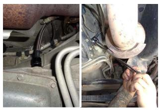
16. Assemble the dipstick tube to the fitting and tighten the nut. **Turn off the vehicle if it is running.**
