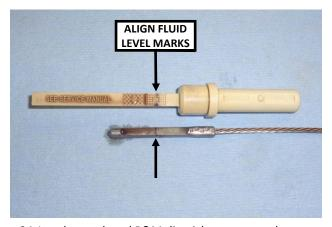
24. Lay the stock and B&M dipsticks next to each other on a bench, and align the two fluid level marks.
