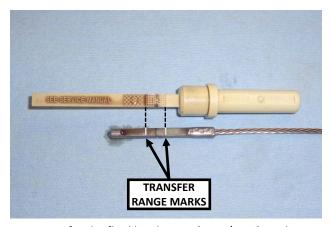
25. Transfer the fluid level range (Max / Min) marks from the stock dipstick to the B&M dipstick. Use a scriber, hacksaw blade or the sharp edge of a needle file to permanently mark the dipstick. Then reinstall the B&M dipstick.
