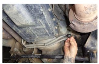
8. Temporarily re-install the stock fill cap, then turn off the vehicle. **NOTE: If the cap is not installed** when the vehicle is turned off, the hot (expanded) transmission fluid may overflow the fill port as it returns to the pan.
