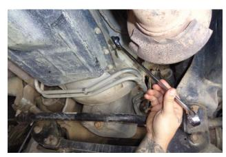
15. Install the dipstick tube fitting (1) in the transmission fill port.
