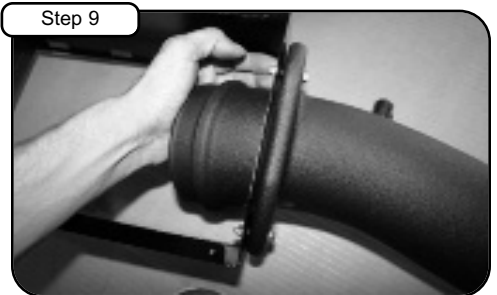
With supplied screws, nuts and washers, mount aFe intake tube onto housing. Tighten using 7/16" socket or wrench.
