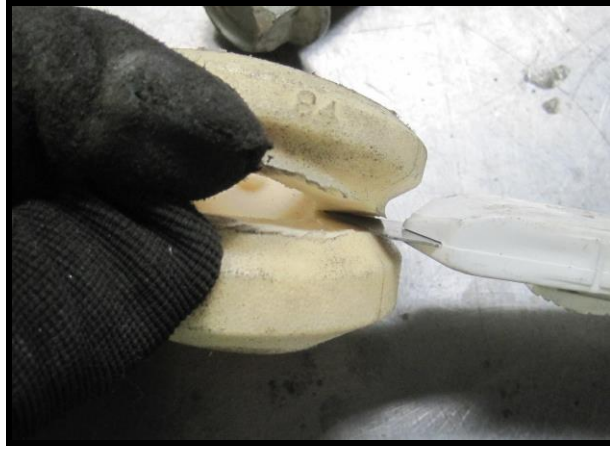
Figure 7- Trimming Front Bump Stop
