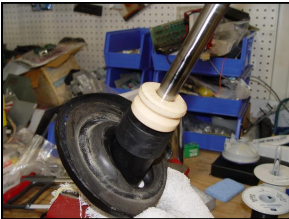
Figure 6 - Front Strut with Boot Removed Exposing Bump Stop
