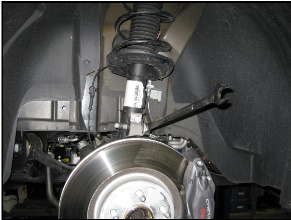
Figure 4 - Removing Spindle to Strut Bolts
