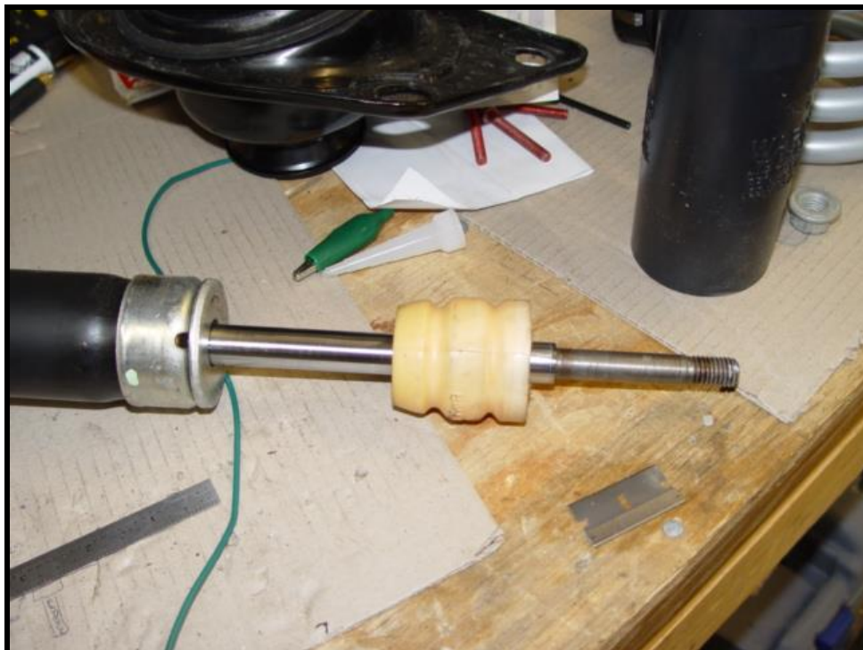
Figure 14 - Strut with un-cut Bump Stop
