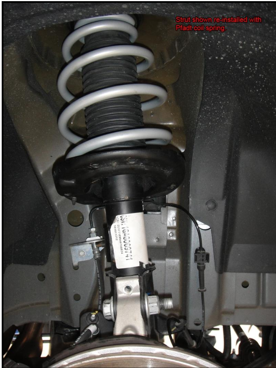
Figure 8 - Front Strut with Pfadt Drop Spring
