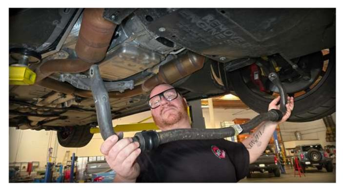
6F Lay out the factory sway bar with the aFe Control sway bar to match the orientation. Lube the inside surface of the bushings with the supplied silicon grease. Install the bushings onto the bar as shown.
