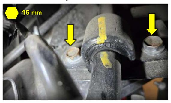
14R You are ready to remove the rear sway bar from the vehicle. Fish the bar ends around the brake line and work your way to the other side. Shown: removing from the driver side.
