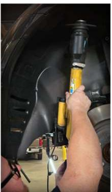
9R Unbolt the end link from the factory sway bar. Repeat on the other side. Retain hardware for reinstallation.
