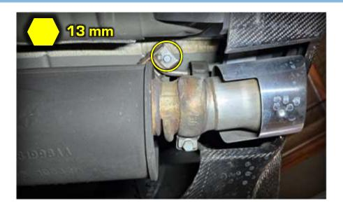
Unbolt the hangers near the rear differential.
