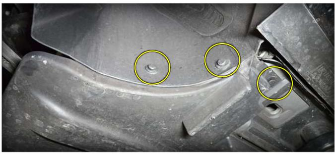
3R Unbolt and remove the (2) tunnel braces.
