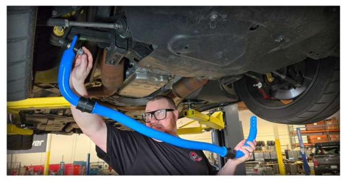
Position the bushing as shown. Don't forget to place the backing plate between the bushing and crossmember as you are reinstalling the bushing bracket.
