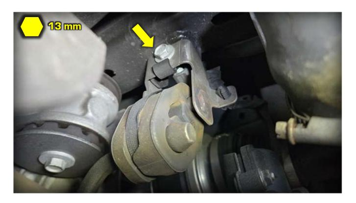
Shimmy the exhaust towards the rear of the vehicle to allow the front pipes to slip out. Remove the exhaust from the vehicle and set aside.
