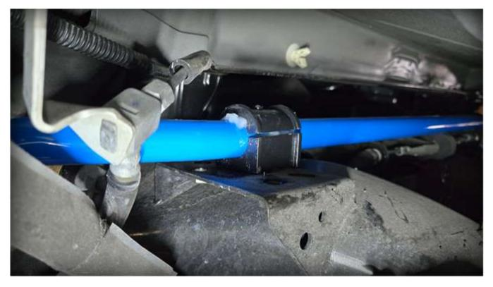
Install the aFe CONTROL billet brackets using the factory bolts. Point the grease fittings outward. Shift the bushing brackets forward when tightening. Torque 45 ft. lbs. This will give the end links the most clearance to the toe link bolt at droop.
