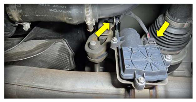
Support the exhaust with a jack and unbolt the hangers near the tips.
