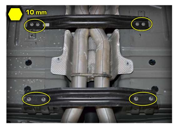
4R The exhaust system will need to be removed or allowed to hang down when we drop the rear crossmember. We removed the exhaust system for clarity.
