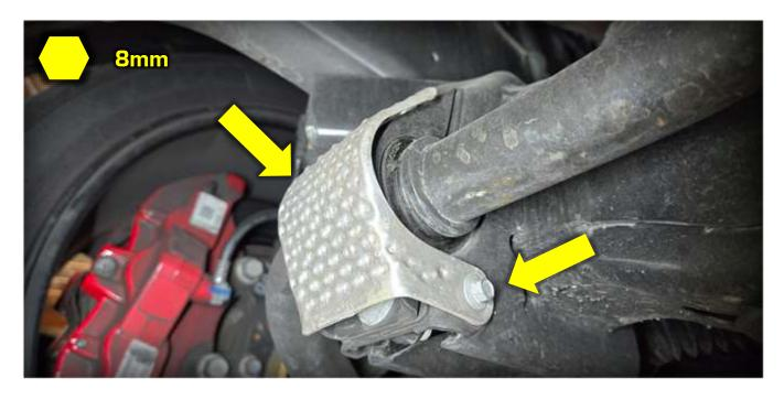
4F Unbolt the bushing bracket (2) bolts per side. Be careful not to lose the back plate that is sandwiched between the bushing and the crossmember.
