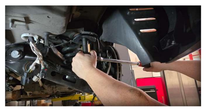
12R Lower the crossmember a few inches and check to make sure no electrical wires or brake lines are pulling.
