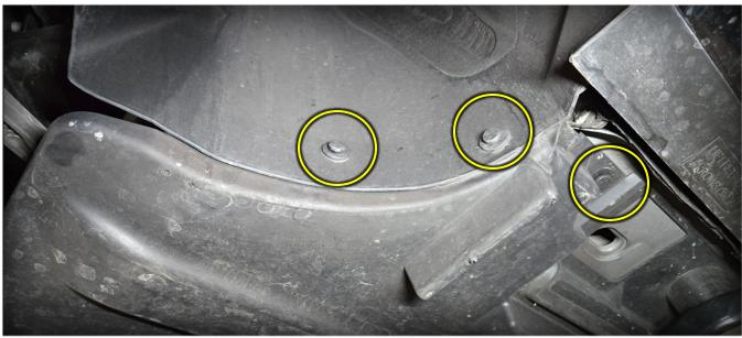
3R Unbolt and remove the (2) tunnel braces.
