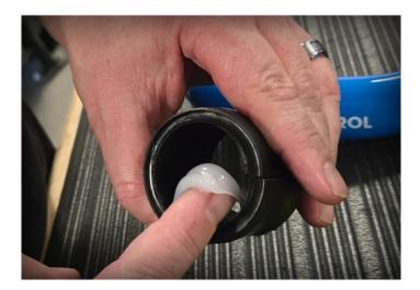
Please Note: Due to the manufacturing process of the bushings, one of the outer surfaces is formed in the mold while the other outer surface is "open" poured. The distance from the center of the bushing to the molded surface is more accurate than the poured side. For this reason, please install the molded side towards the sway bar centering ring.
