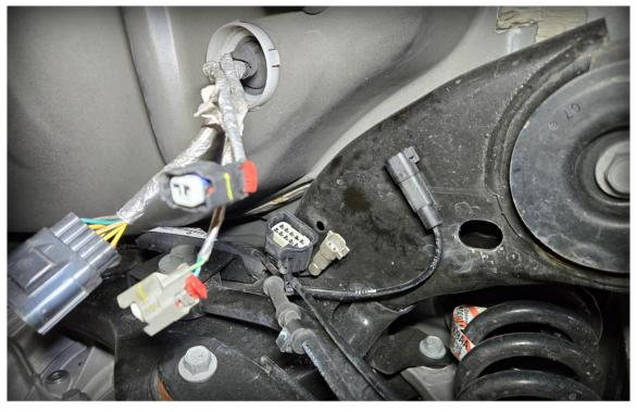
6R Work your way over to the fender-well area and unfasten (2) nuts and (3) pop clips to access the brake line bracket. Peel back the fender well and unfasten the bracket from the body. Do this to both sides.
