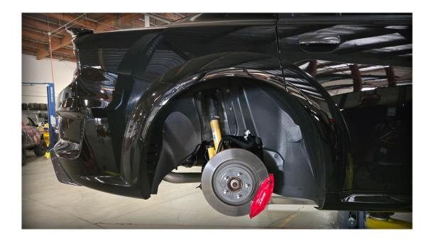
2R Unbolt the (7) bolts and (3) pop clips to remove the rear plastic under tray. Perform on both sides.
