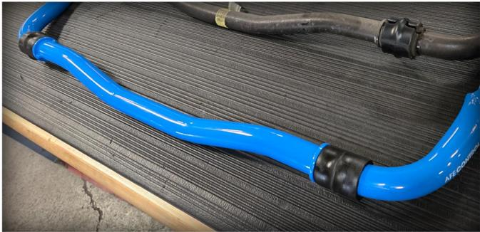
Reinstall the sway bar in the same manner as removal. Start with the end links to help hold the bar in place. The hole furthest from the end is the stiffest setting. (Shown) The hole closest to the end is the softest setting. Spin the nuts on finger tight for now.
