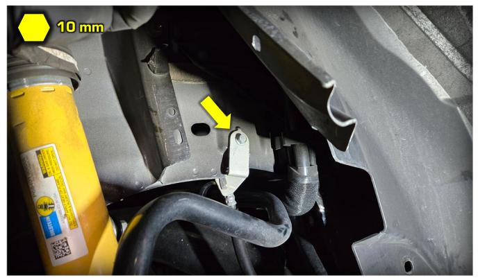
7R Continuing with the brake lines, follow the line inward over the top of the crossmember and unclip the line from the white clip. Do this to both sides.
