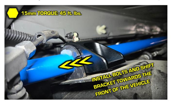
17R Fully tighten the factory bolt/nut onto the sway bar end. The hole furthest from the end is the stiffest setting. The hole closest to the end is the softest setting. Tip: Add some thread locking compound to the end link stud to ensure long lasting tightness. Torque: 45 ft.lbs.
