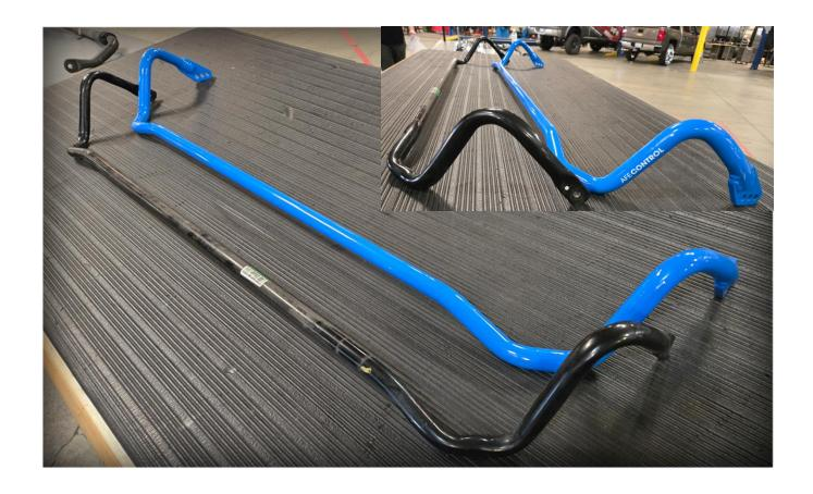
15R Reapply the poly bag back onto the aFe CONTROL sway bar for protection and install the sway bar in the same manner as removal. Remove bag after is in position.
