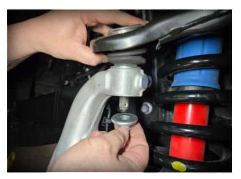
Push the knuckle towards the rear of the car but do not pull outward to avoid pulling the CV joint out of its cage.
