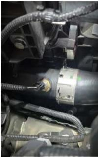
Unclip the retaining clip and disconnect the charge pipe. (View from underneath)
