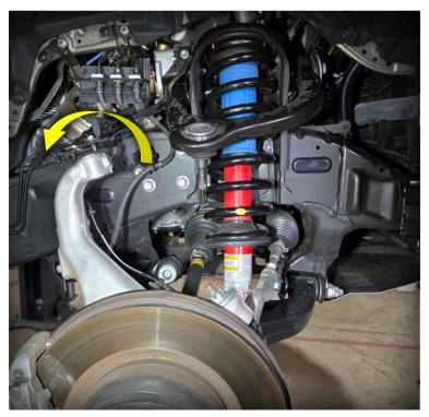
Slide the cross bolt toward the front and remove the passenger side arm.
