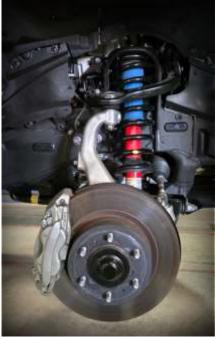
Disengage the ABS line from the factory upper control arm retention clips. Use a slotted screwdriver and carefully pry the clamps open.
