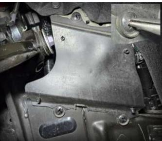
Passenger Side: The cross bolt will need a few things moved out of the way before it can be removed from the frame mount.
