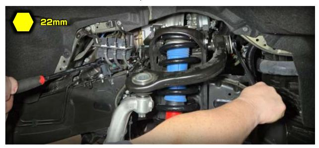
Fully remove the castle nut and disengage the upper control arm from the knuckle.
