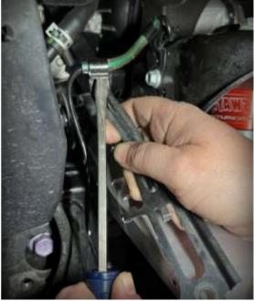
Remove the factory cotter pin using a pick. Loosen but do not remove the castle nut. Leave about a  $\frac{1}{4}$ " of gap between the knuckle mount and nut.
