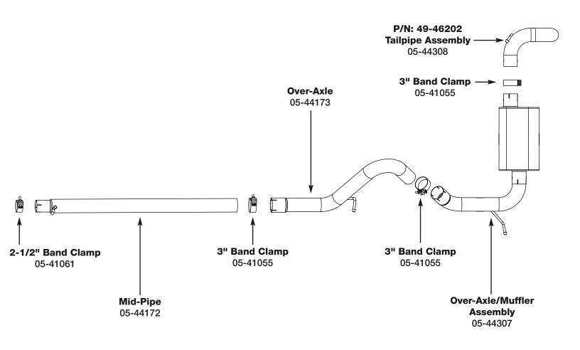
**Step 1:** (Read Instructions prior to installation) Remove your stock exhaust from the rear of your jeep working your way forward. It may be necessary to cut the pipes if the slip joints are stuck. Take caution not to damage the factory isolation mounts as they will be reused. It is recommended to not fully tighten the clamps until the entire system has been installed.
