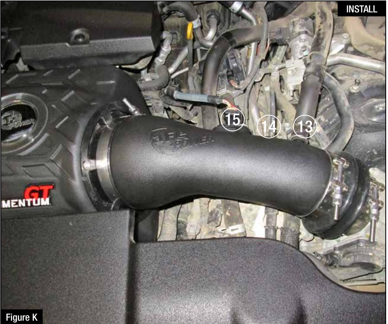
**Figure K****Refer to Figure K for Steps 13-14**
