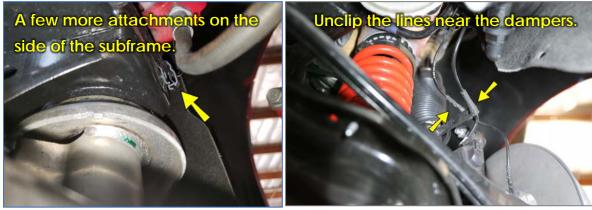
Unclip the electronic damper connector for each rear shock.
