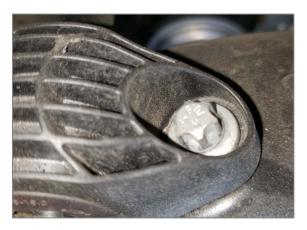
17R Remove the factory sway bar from the left side of the vehicle. Note the orientation of the sway bar when removing. (i.e. observe which is the top of the sway bar and how the ends are pointing.)
