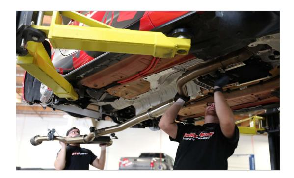
6R Undo the plastic nuts to remove the heat shield (10mm socket)
