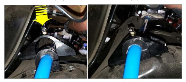
22R Reattach the end links to the sway ends reusing the factory nuts. The hole closest to the end is the soft setting. Settings get stiffer as you move away from the ends. (optional: apply thread locking compound to the end link thread)
