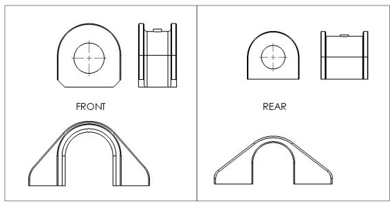
9F Install the front aFe Control sway bar in the same manner as factory removal. Place the factory base plate up to the subframe studs. Slide the aFe Control bushing bracket onto the bushings and mate the sway bar assembly to the subframe. Reuse the factory nuts to secure the brackets to the subframe. Fully tighten this hardware to factory specs.
