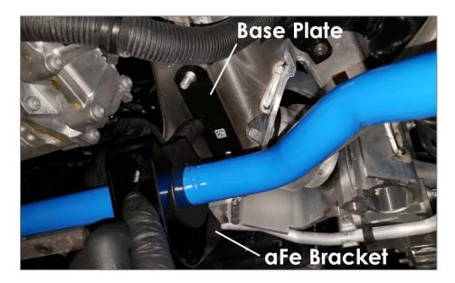
10F Reattach the end links to the sway bar ends reusing the factory nuts. The hole closest to the end is the softest setting. Settings get stiffer as you move away from the ends. (optional: apply thread locking compound to the end link thread)
