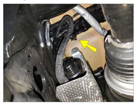
11R Unbolt the lower shock mounts. (18mm socket & wrench)
