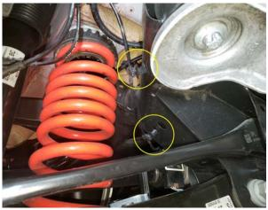
10R Detach the harness clip attaching the active differential wires to the subframe on the right side of diff.
