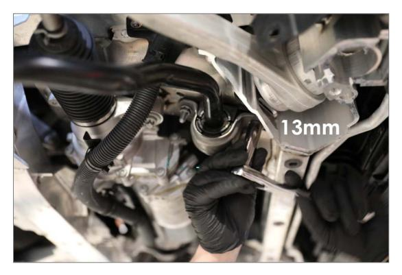
Remove the factory sway bar from the vehicle. Note the orientation of the sway bar when removing. (i.e. observe which is the top of the sway bar and how the ends are pointing.)
