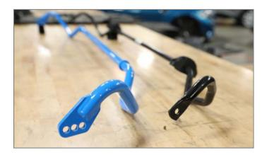
19R Grease the rear bushings with the supplied silicone lube and install bushings onto the sway bar. The bushings should be positioned just outside of the centering rings.
