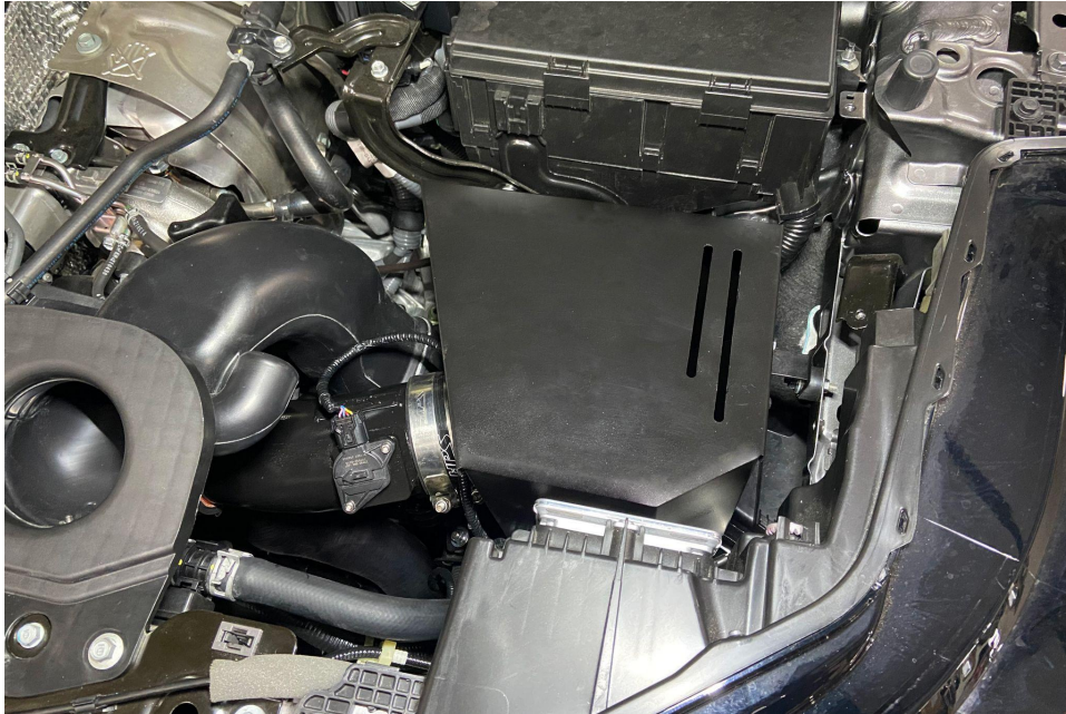
19. Secure the heat shield lid with the provided M5x12mm bolts (4).
