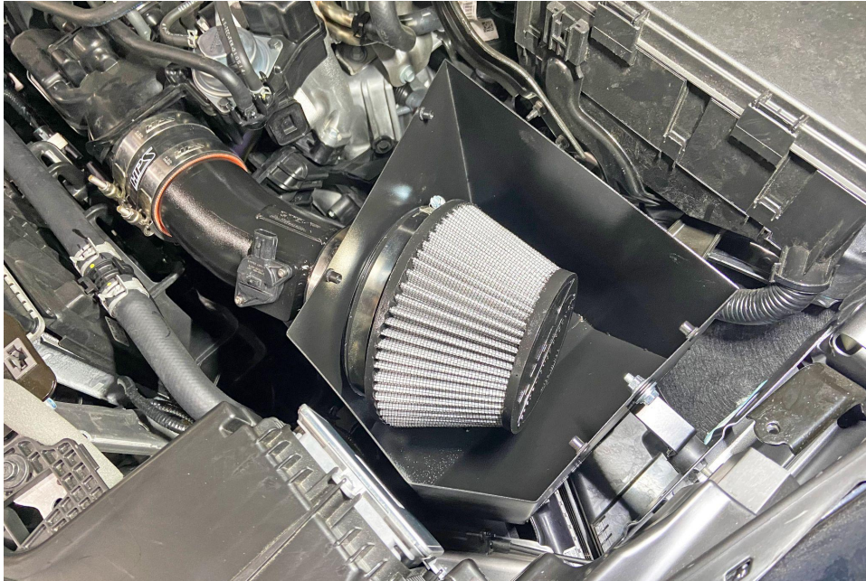
15. Install the HPS performance air filter onto the velocity stack.
