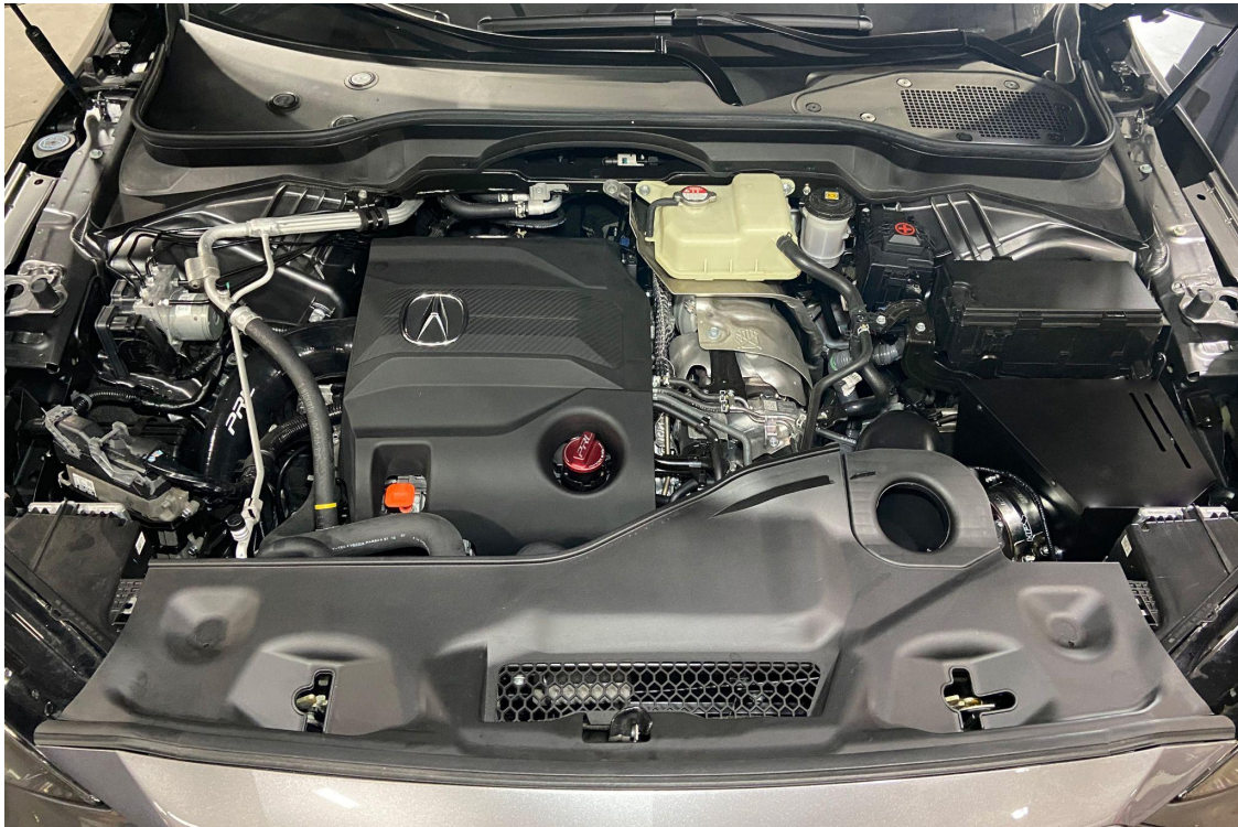
20. Reinstall the radiator cover panel onto the vehicle.
