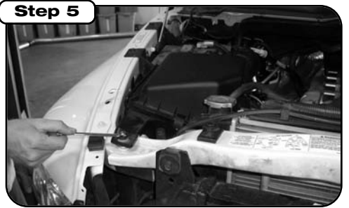
Step 5 Using 10 mm wrench, remove the bolt that secures the factory airbox to the radiator bulkhead.
