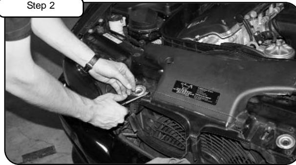
Remove inlet duct retaining pins and inlet duct.
