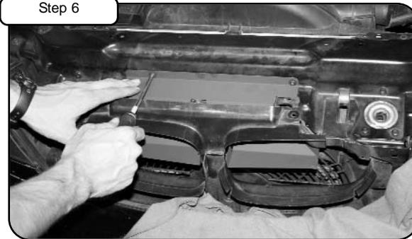
Replace the screws removed in step 3.
