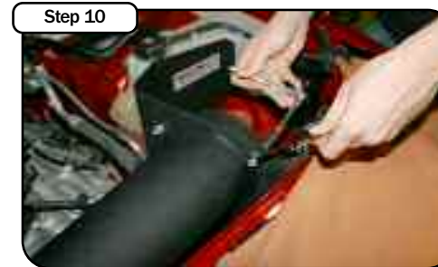
Align the mounting holes on the tube and the housing. Secure the assembly with the provided M6 bolts washers and nuts.
