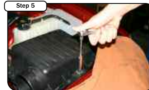
Remove the 10mm screw securing the airbox to the vehicle. Save for re-use later.
