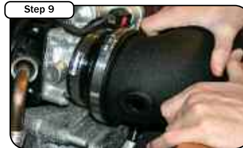
Place coupler and hose clamps on the throttle body. Position tube into coupler and tighten the clamps down.
