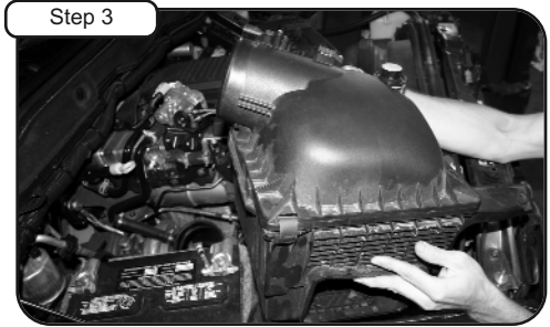
Step 3 Disconnect air temp sensor. (6.7L, disconnect MAF sensor). Lift up and pull OE air box out of vehicle.
