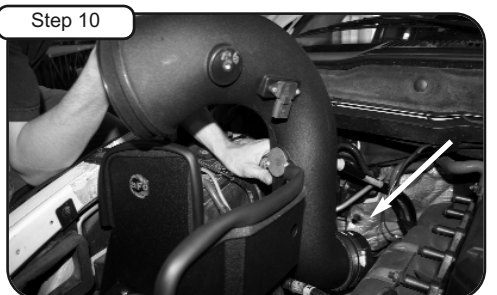
Step 10 Install hi-temp coupler with clamps provided to tube. Now install tube into vehicle.
