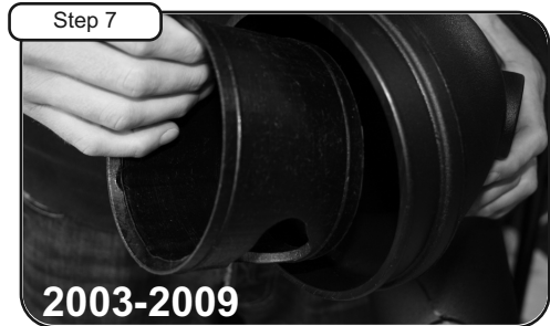
Step 7 For trucks before 2010, remove MAF insert coupling from inside tube. (Keep for 2010-2011 trucks to prevent check engine light.)
