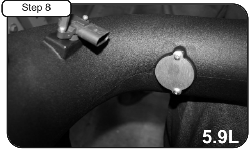
Step 8 With T-20 torx bit remove temp sensor and (with gasket and screws provided) install into new tube. (5.9L place MAF cover with gasket and tighten using short screws provided. Install plug into the hole in tube for crank case line.)
