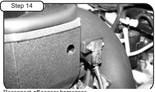
Step 14 Reconnect all sensor harnesses.
