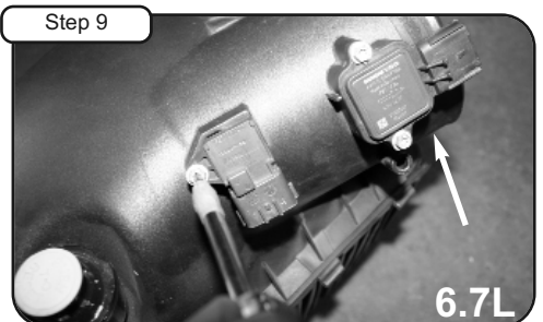
Step 9 (6.7L remove and install temp sensor, see step 7) 6.7L, remove MAF sensor and install to new tube with screws and gasket (Make sure gasket is between sensor and tube) Install grommet only to tube. The 6.7L will not use small phillips screws.
