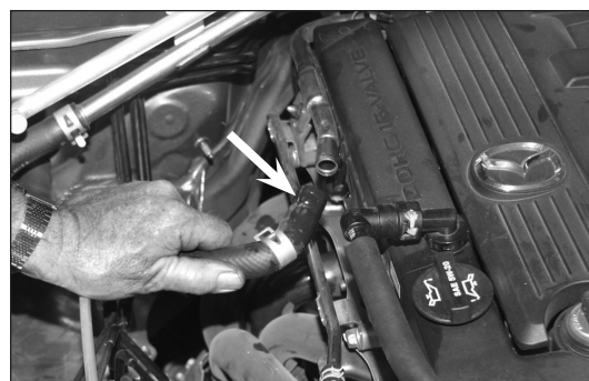
Figure B - Remove the heater hose.
