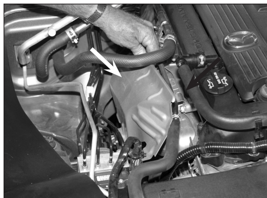
Figure A - Remove the upper and lower heat shields.
