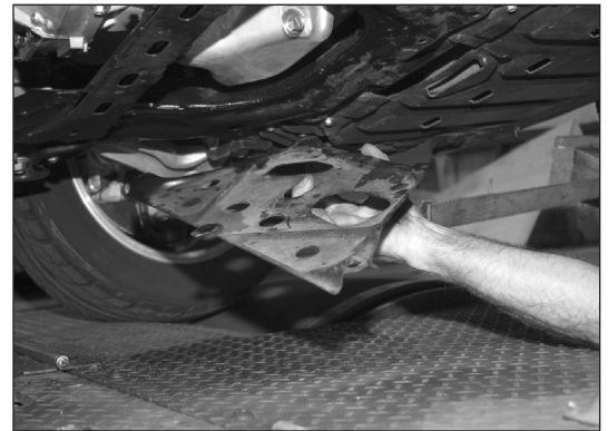
Figure F - Remove the cover plate.
