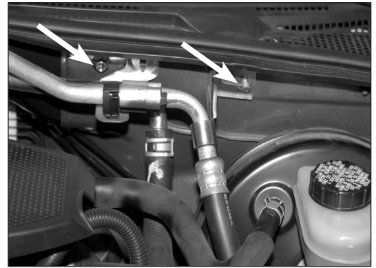
Figure E - Remove the retaining nuts.
