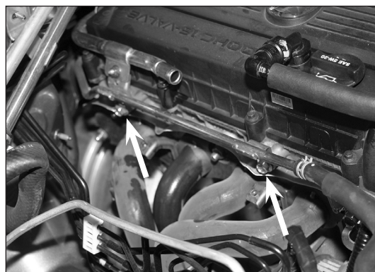
Figure D - Remove the coolant line retaining bolts.
