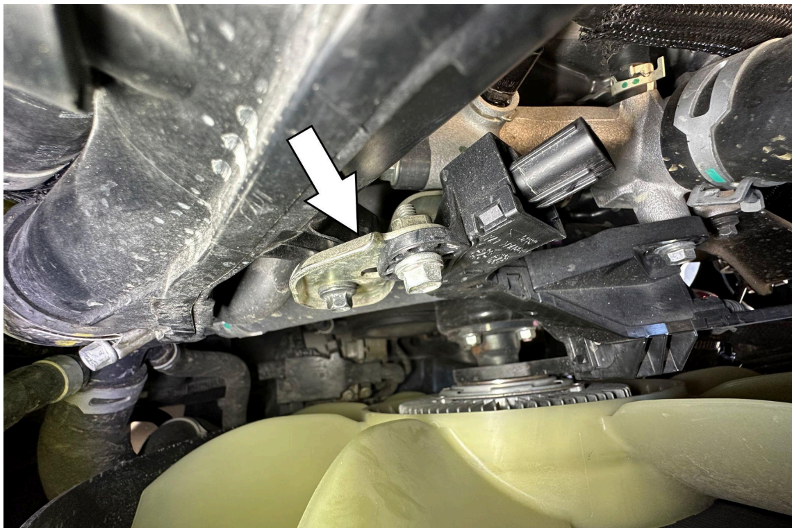
8. Remove the two mounting bolts and mounting bracket on the passenger side charge pipe.
