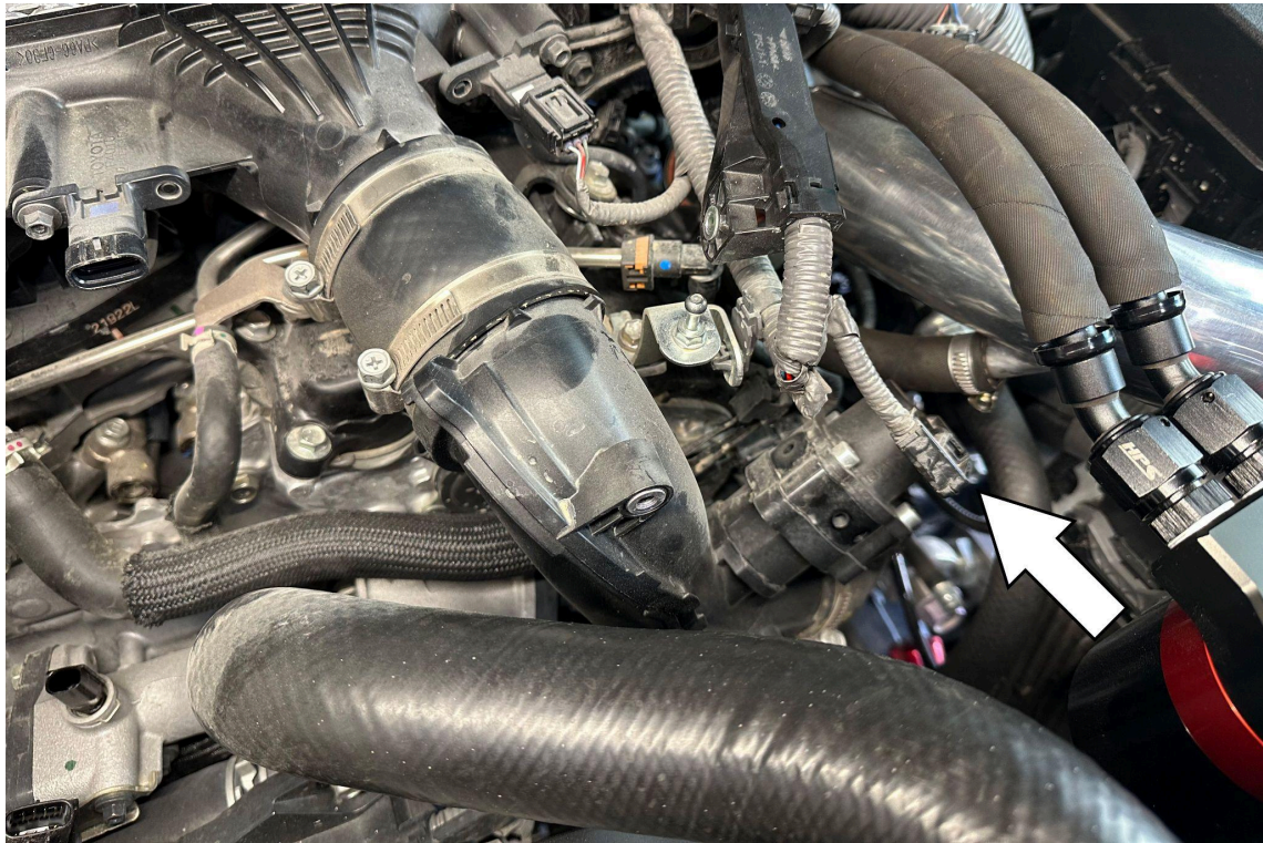
5. Disconnect the harness connected to the blow off valve on the driver side.
