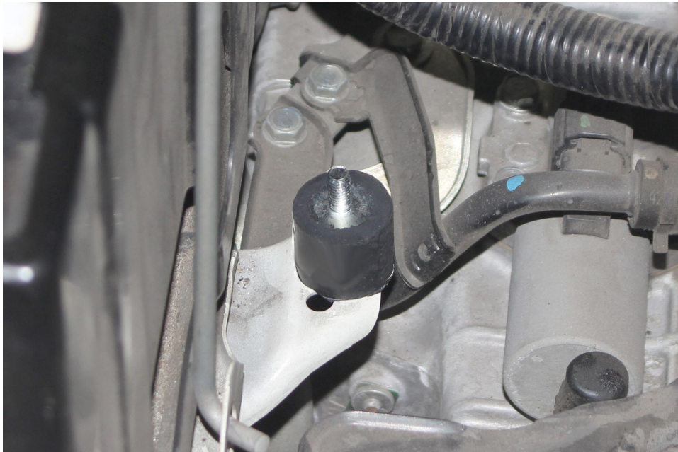
10. Install the 1" tall rubber vibration mount onto the factory air box mount located behind the battery.
