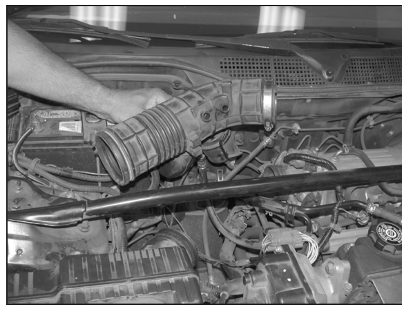
4. Loosen the hose clamp at the throttle body, then, remove the stock intake tube as shown.
