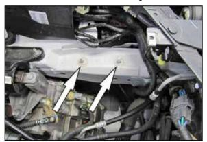
9. Remove the two air box mounting studs shown from the inner fender.
