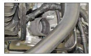
11. Install the provided silicone hose (084016) onto the throttle body and secure with the provided hose clamp.
