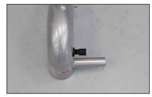
18. Install provided grommet and factory inlet air temperature sensor into the K&N® intake tube as shown.
