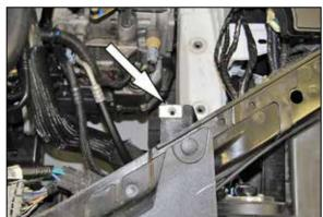
10. Remove the air box mounting clip nut from the core support.
