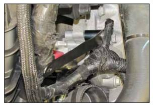
13. Install the tube mounting bracket (064307) as shown using the provided hardware.
