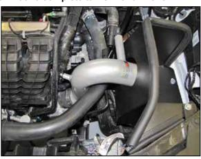
20. Install the K&N® intake tube into the heat shield and silicone hose at the throttle body, align with the mounting bracket and then secure with the provided hardware.
