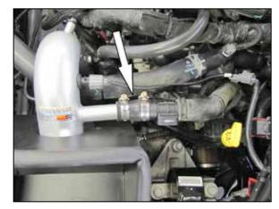
23. On vehicles equipped with air injection, connect the air injection hose to the K&N® intake tube using the provided coupling hose and clamps. On vehicles that are not equipped with air injection, install the provided cap and secure with the provided hose clamp.
