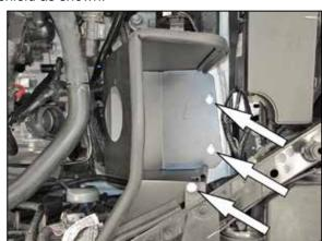
16. Install the heat shield onto the inner fender and secure with the provided hardware.
