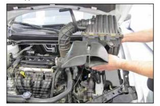
8. Remove the factory intake and air filter assembly from the vehicle.
