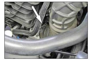
6. Loosen the hose clamp that secures the factory intake hose to the throttle body and then disconnect the intake hose from the throttle body.
