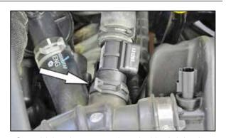
5. On vehicles that are equipped with air injection, release the spring clamp securing the air injection hose and then disconnect the air injection hose from the factory intake tube.
