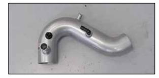
19. Install the  $90^{\circ}$  vent fitting into the K&N® intake tube as shown.
