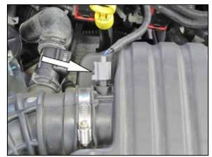
4. Disconnect Inlet air temperature sensor electrical connection.
