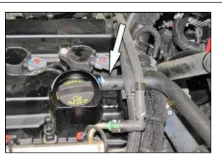
3. Disconnect the crank case vent hose from the valve cover port.
