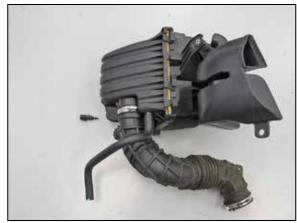
17. Remove the inlet air temperature sensor from the factory air box.
