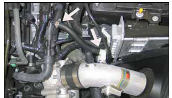
24. Install provided silicone hose onto the EVAP valve with provided hose clamp then onto 90° fitting on K&N® intake tube. NOTE: Some trimming maybe necessary.
