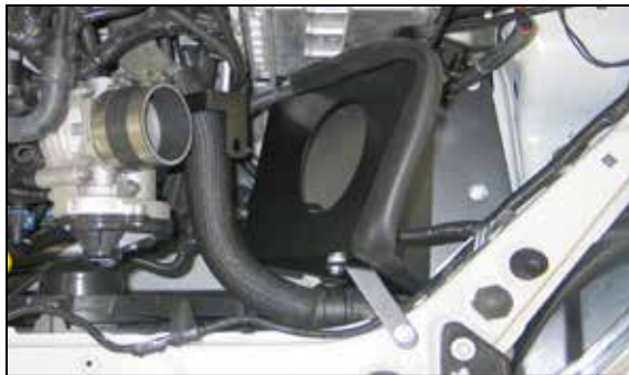
18. Install the heat shield into the vehicle as shown and secure with the provided hardware and the bolt removed in step #10.
