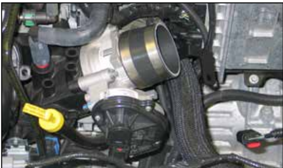
13. Install silicone hose (08440) with provided hose clamps onto the throttle body as shown.
