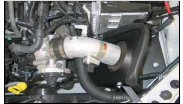
23. Install K&N® intake tube into silicone hose and aligning with tube mounting bracket and heat shield. Secure with provided hardware as shown.
