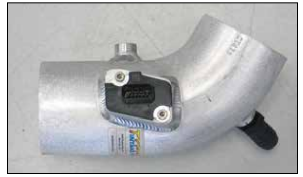
22. Install mass air sensor into K&N® intake tube and secure with the provided hardware as shown.
