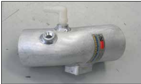
19. Install 90 degree vent fitting into the K&N® intake tube as shown. NOTE: Plastic NPT fittings are easy to cross thread. Install the vent fitting "hand" tight, then turn it two complete turns with a wrench.
