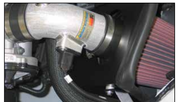
27. Attach mass air extension harness onto factory harness and connect the other end to the mass air sensor electrical connector.
