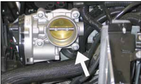
11. Remove bolt shown from throttle body. NOTE: bolt will be reused.
