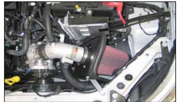
26. Install the K&N® filter onto K&N® intake tube secure with provided hose clamp as shown. NOTE: Drycharger® air filter wrap; part # RX-4990DK is available to purchase separately. To learn more about Drycharger® filter wraps or look up color availability please visit http://www.knfilters.com ®.
