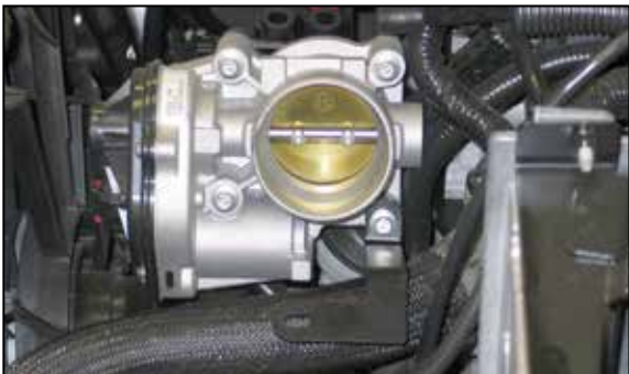
12. Install tube mounting bracket (083136) onto the throttle body using bolt removed from the previous step.
