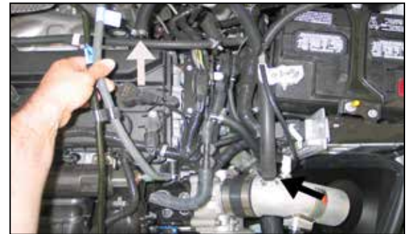
25. Install provided silicone hose at rear of cam cover and secure with provided hose clamp, then install the other end of the hose onto the 5/8" fitting on K&N® intake tube as shown. NOTE: Some trimming maybe necessary.
