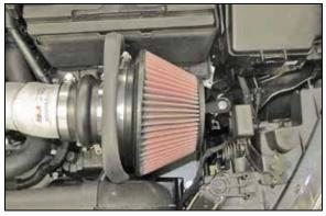
19. Install the K&N® air filter and secure it with the hose clamp provided.
