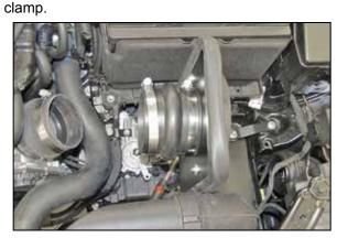
15. Install the hump hose (5-576) onto the filter adapter and secure with the provided hose clamp.
