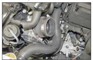
14. Install the provided hump hose (08421) onto the throttle body and secure with the provided hose
