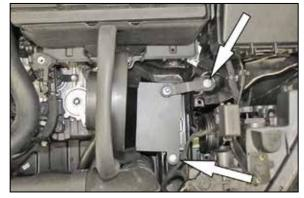
13. Install the heat shield onto the inner fender and secure with the provided hardware as shown.
