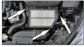
6. Loosen and remove the three bolts securing the lower air box to the inner fender.
