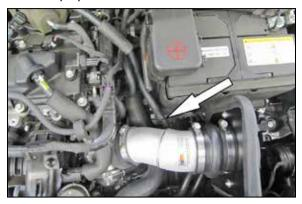
18. Connect the factory crank case vent hose to the fitting installed into the K&N® intake tube and secure with the factory hose clamp.
