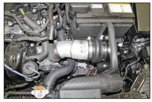
17. Install the K&N® tube into the hose at the filter adapter and then into the hose at the throttle body, then adjust the tube for best fit and secure with the hose clamps provided.
