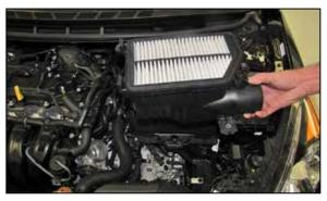
7. Remove the lower air box from the vehicle.
