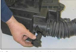
13. Remove the two bolts which secure the mass air sensor to the factory airbox and then remove the mass air sensor as shown.
