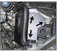
12. Install the heat shield assembly onto the inner fender and secure with the factory bolts removed during steps #6 and #7.
