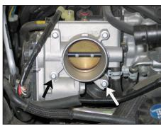
8. Remove the two lower throttle body mounting bolts shown.
