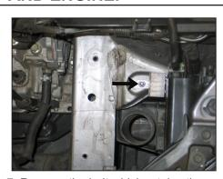
7. Remove the bolt which retains the ground strap to the inner fender.
