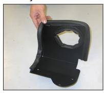
11. Install the provided short edge trim into the hole of the heat shield as shown.
