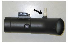
15. Install the provided vent fitting into the K&N® intake tube as shown.
