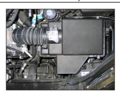
4. Loosen the hose clamp which secures the intake tube to the throttle body.
