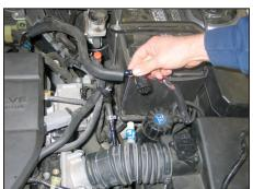
3. Disconnect the crankcase vent hose from the intake tube as shown.
