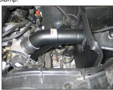
18. Install the K&N® intake tube into the silicone hose at the throttle body and align with the tube mounting bracket. Secure the intake tube with the provided hose clamp and hardware.
