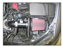
20. Install the K&N® air filter onto the K&N® intake tube and secure with the provided hose clamp. NOTE: Drycharger® air filter wrap; part #RX-4730DK is available to purchase separately. To learn more about Drycharger® filter wraps or look up color availability please visit http://www.knfilters.com®.
