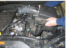
5. Pull up firmly on the airbox assembly to dislodge it from the mounting grommets and then remove the airbox assembly from the vehicle.
