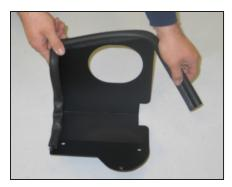
10. Install the provided long edge trim onto the heat shield as shown.
