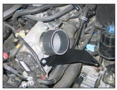
17. Install the silicone hose (08440) onto the throttle body and secure with the provided hose clamp
