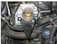
9. Install the intake tube mounting bracket onto the throttle body and secure with the original bolts removed in the previous step.
