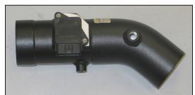
14. Install the mass air sensor into the K&N® intake tube and secure with the provided hardware.
