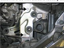
6. Remove the two bolts which secure the airbox mounting bracket to the inner fender and then remove the bracket from the vehicle.
