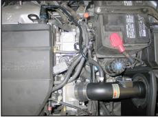
19. Install the provided crankcase vent hose onto the factory vent tube and onto the vent fitting installed into the K&N® intake tube as shown.
