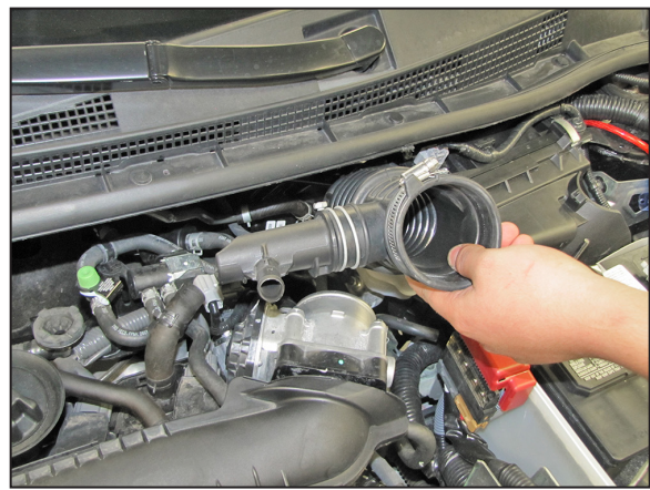
5. Remove the intake hose from the vehicle.
