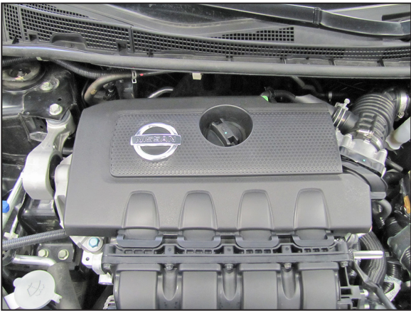
2. Lift up and remove the engine cover.
