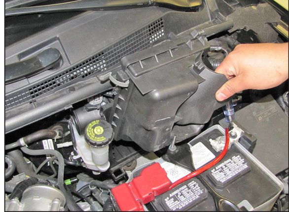
6. Release the two air box clips and then remove the front half of the air box and air filter.
