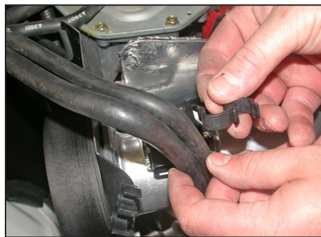
22. Remove the coolant hose clip as shown.
