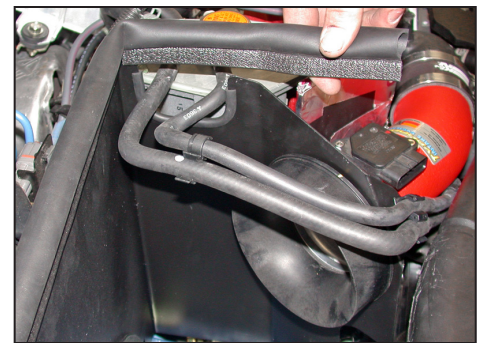
28. Install the remaining trim seal onto the heat shield and trim to fit as shown. NOTE: Some trimming of the edge trim may be necessary.
