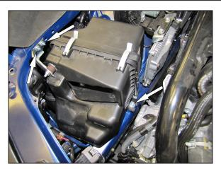
3. Remove the two nuts that secure the air box bracket to the inner fender and the bolt that secures the air box to the frame rail.
