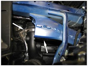
6. Loosen the hose clamp that secures the factory intake tube to the factory turbo inlet tube and remove the nut mounting the tube to the frame. NOTE: the nut is under the frame member. This nut will be reused in a later step.
