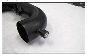
9. Install the provided rubber mounted stud onto the K&N® intake as shown.
