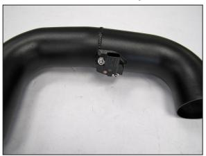
8. Remove the mass air sensor from the Factory intake tube and install it in to the K&N® intake tube using the provided hardware.
