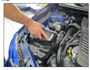
4. Release the two retaining clips and then remove the front half of the air filter housing and the factory air filter.
