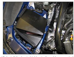
16. Install the heat shield onto the rubber mounted stud and the studs on the inner fender, secure with the factory nuts and hardware.
