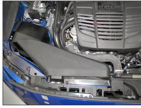
17. Reinstall the fresh air intake scoop so the outlet engages with the heat shield then secure with the factory retaining clips.
