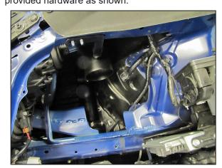
11. Install the K&N® intake tube into the factory turbo inlet tube, align the bracket with the studs on the inner fender and then secure with the hose clamp provided.
