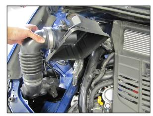
7. Separate the intake tube from the turbo inlet tube and remove the complete assembly from the vehicle.
