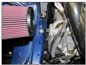
13. Install the K&N® air filter onto the intake tube and secure with the provided hose clamp. Install the provided rubber mounted stud onto the frame in the factory air filter housing mounting location as shown.
