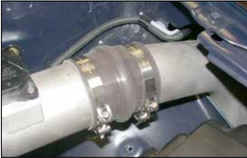
26. Slide the K&N® cold air tube through the inner fender from underneath the vehicle and insert the tube into the silicone hump hose as shown above. **NOTE: Before installing the intake tube, inspect the inside of the tube for any debris, then clean the inside out with water and a towel. Inspect the tube one more time before proceeding to the next step.**
