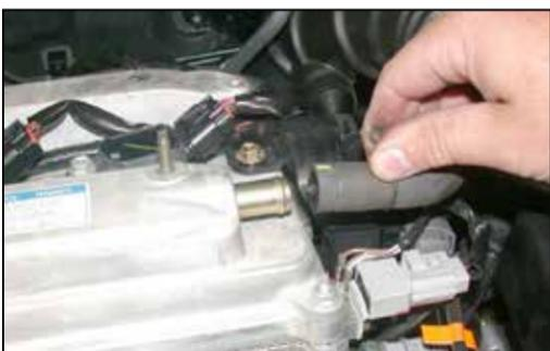
3. Remove the crank case vent hose from the cam cover as shown.
