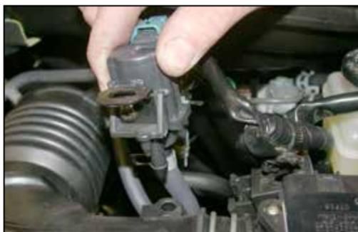
6. Using a flat blade screwdriver pry up the vacuum switching valve from the stock intake tube as shown.
