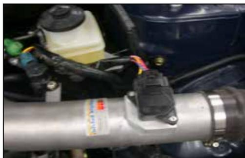
36. Reconnect the mass air sensor electrical connection as shown.
