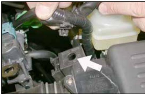
5. Unclip the wire harness from the air cleaner assembly as shown.
