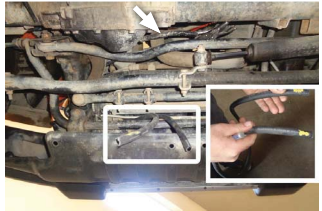
15. Trim cooler hose long enough to splice into return hose line. Mark both ends of remaining line then route it back through to super cooler.
