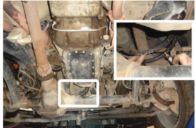
14. Identify and mark factory transmission return line.
