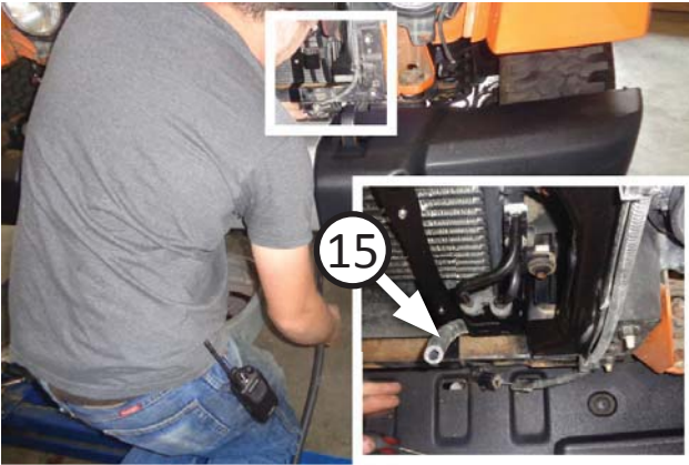
11. Route \frac{3}{8} " transmission oil cooler hose (15) through driver side corner of grill frame from underside of vehicle.
