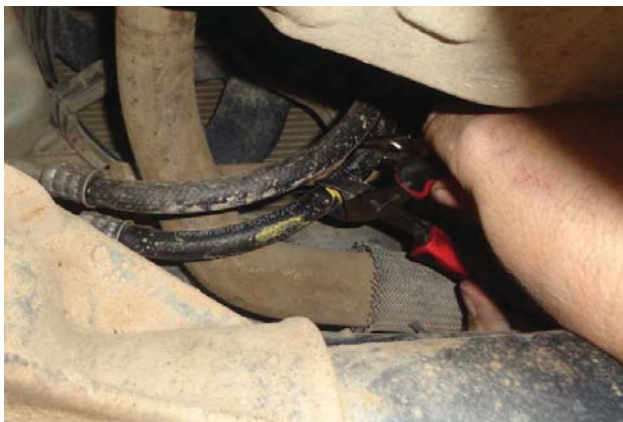
18. Isolate trim location on return line with vice grips. Route cooler hoses over to return line.
