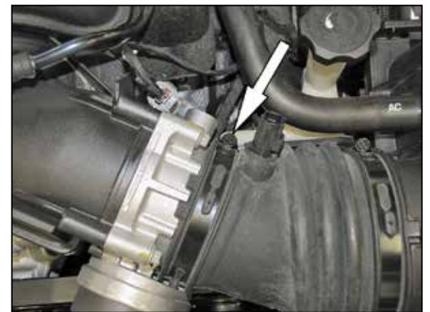
5. Loosen the hose clamp securing the intake tube to the throttle body.
