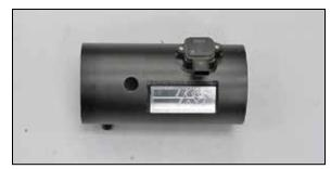
14. Install the mass air sensor into the K&N® intake tube and secure with the provided screws.
