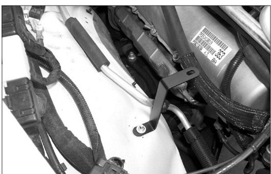
10. Mount the provided "Z" bracket onto the inner fender well as shown. Do not tighten completely.
