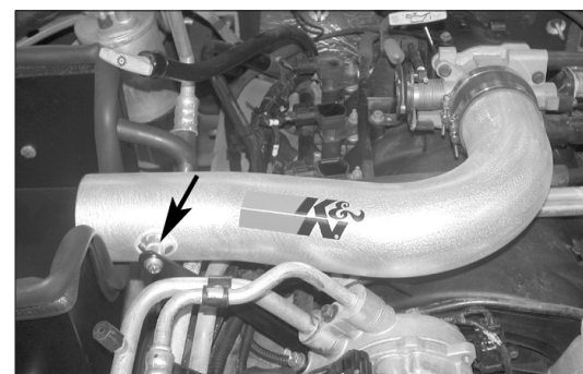
21. Install the K&N® intake tube onto the throttle body and secure with the provided hose clamp, then secure to the tube mounting bracket installed in step #19 with the provided hardware as shown.
