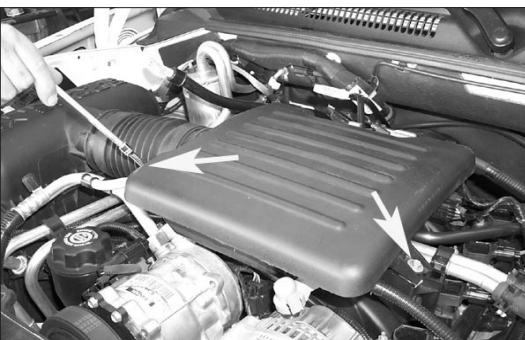
3. Loosen and remove the two bolts that retain the air resonator to intake manifold as shown.
