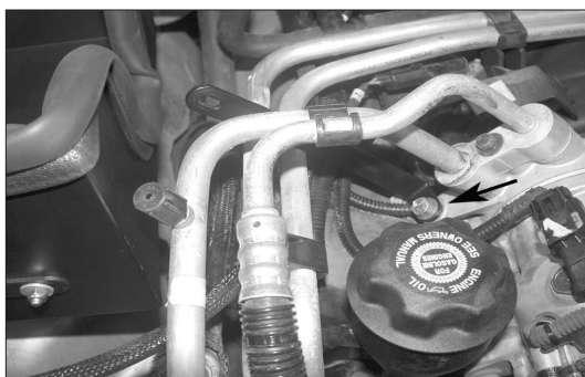
19. Install the tube-mounting bracket onto the A/C compressor with the bolt removed in step #18.
