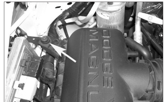
6. Loosen and remove nut that retains airbox to vehicle.
