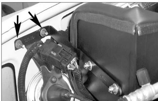
15. Using the nuts that was removed in step 13, secure the bracket to the inner fender well.
