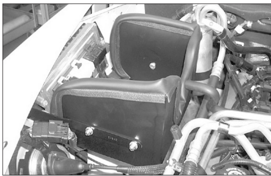
14. Install the heat shield into the vehicle as shown.
