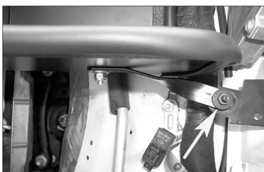
16. Using the nut that was removed in step 6, secure the bracket to the airbox mounting stud as shown. Do not tighten at completely at this time .
