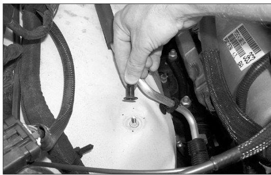
8. Unscrew plastic airbox retaining stud from vehicle as shown.
