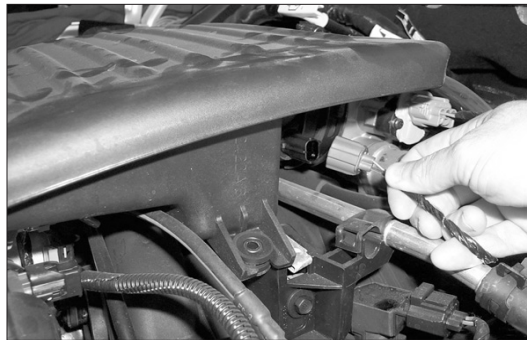
3a. On vehicles that come equipped with an air temp sensor, disconnect the electrical connection as shown.
