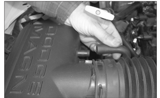
5. Remove vent hose from airbox as shown.
