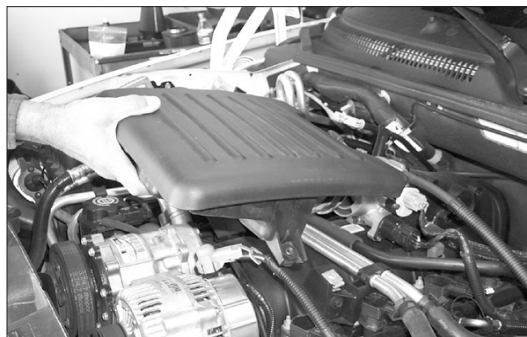
4. Remove the air resonator from vehicle as shown.
