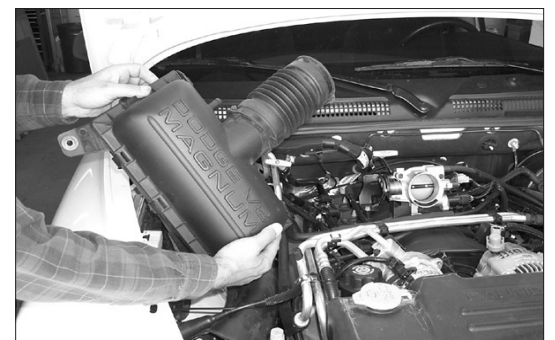
7. Pull firmly upwards on stock airbox to remove from vehicle as shown. NOTE: K&N Engineering, Inc., recommends that customers do not discard factory air intake.
