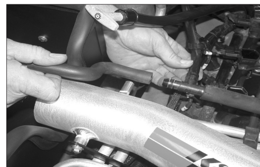
22. Remove the vent hose from vehicle as shown.
