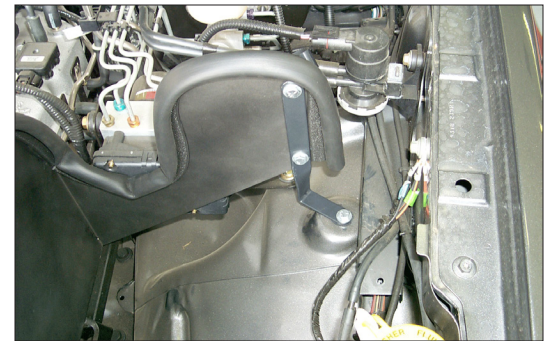
8. Install the heat shield into the vehicle and secure the twist bracket to the original air cleaner mounting hole using the provided hardware.
