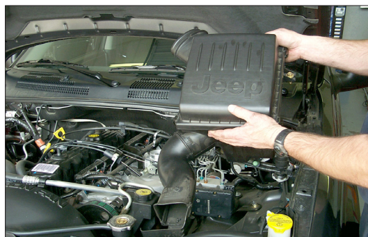
5. Remove the three nuts that secure the air cleaner assembly from underneath the vehicle, then, remove the air cleaner assembly as shown. NOTE: K&N® recommends that you do not discard your factory air intake.
