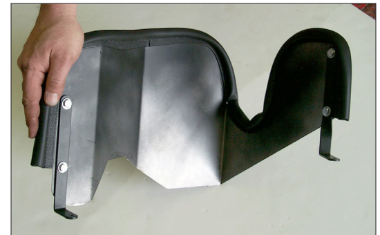
7. Using the provided hardware install the two brackets onto the heat shield as shown.
