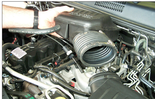
4. Loosen the hose clamp at the air cleaner lid and at the throttle body, then, remove the resonator and bellows assembly as shown.
