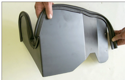
6. Install the provided trim seal onto the heat shield as shown. NOTE: Some trimming of the edge trim will be necessary.
