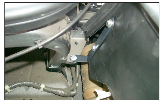
9. Secure the "L" bracket to the hole on the flange/tab on the radiator core support using the provided hardware.
