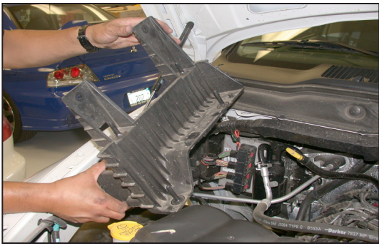
10. Remove the air cleaner support bracket which is held in place by four bolts.
