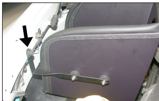
20. Secure the twist bracket to the threaded hole on the inner fender using the original hex bolt from step 10.
