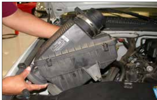
6. Pull firmly upwards to remove the air cleaner assembly as shown. NOTE: K&N Engineering, Inc., recommends that customers do not discard factory air intake.
