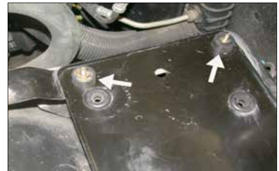
9. Install the rubber mounted studs as shown and tighten firmly.
