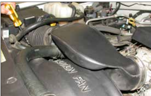
3. Loosen the hose clamps at the throttle body and at the mass air sensor.
