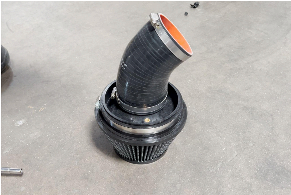
18. Secure the HPS air filter onto the velocity stack. Then, secure the 45 degree coupler using the provided EMSC clamps onto the outlet side of the velocity stack.
