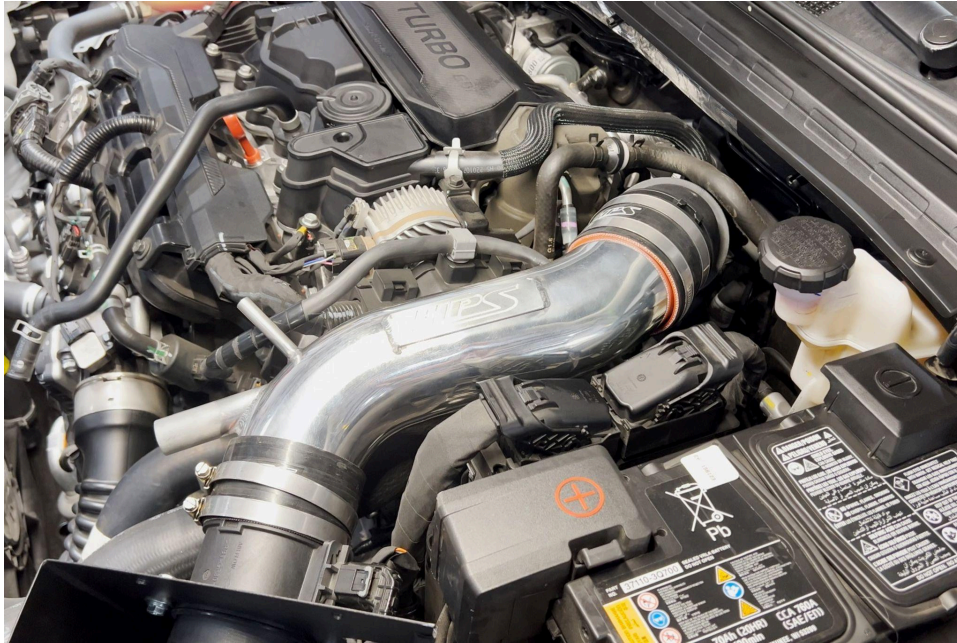
17. Insert and secure the HPS intake pipe into the couplers.
