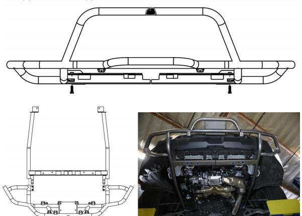
9. If Installing 79-27009 the installation is complete. If installing 79-27012 with the winch proceed to install the Skid Plate using the (2) 3/8-16 Bolts, (2) 3/8 Washer, (2) M8 Bolts, & (2) M8 Nuts.
