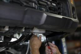
5. On the underside of the vehicle remove the (10) Bolts. Remove the front under guard from the vehicle.
