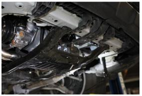
6. Install the Passenger Side Bumper using the (2) M8 Bolt, (2) M8 Flat Washer, (2) M8 Lock Washer, (1)1-1/8" Washer, and (2) O.E. Bolts. Sandwich the Under Guard between the Frame and the Bumper When Tightening Down the Hardware.
