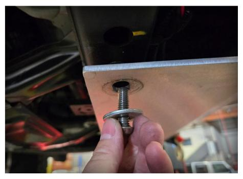
If you do not have our front skid plate, Install the button head bolts and washers onto the bumper crossmember's 3/8 rivnut holes. Leave loose with about a  $\frac{1}{4}$ " gap between the washer and the bumper crossmember.
