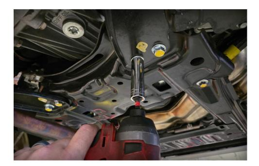
5. Install the aFe spacers using the included longer M10 flanged bolts. Fully tighten.
