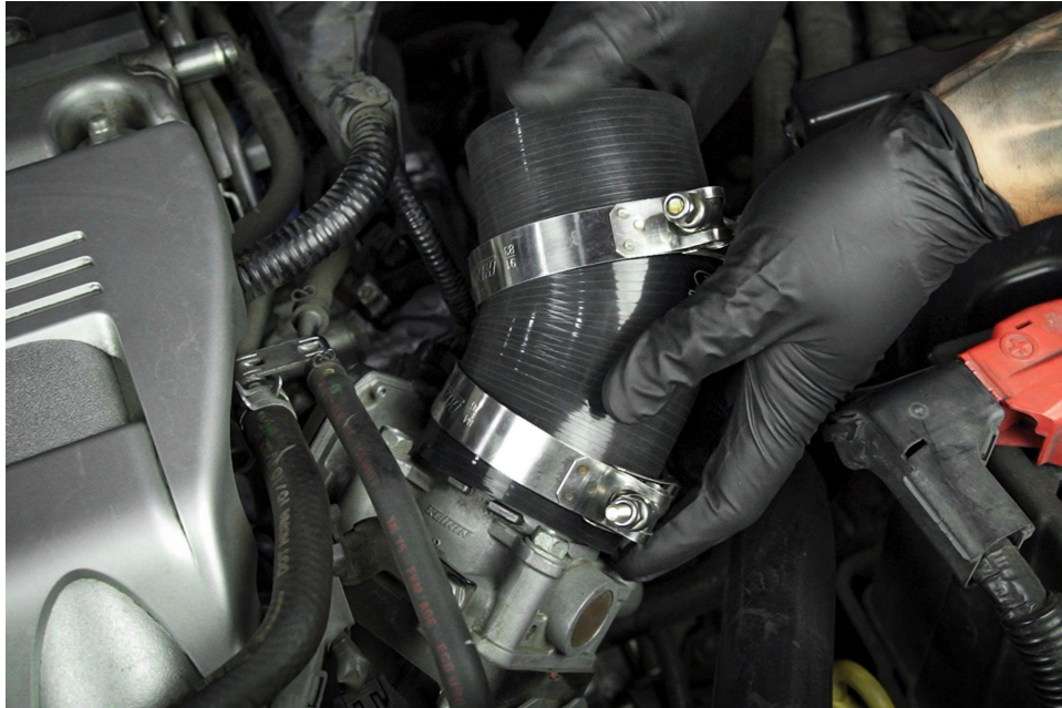
13. Install the 45 degree coupler along with the provided T-bolt clamps onto the throttle body.
