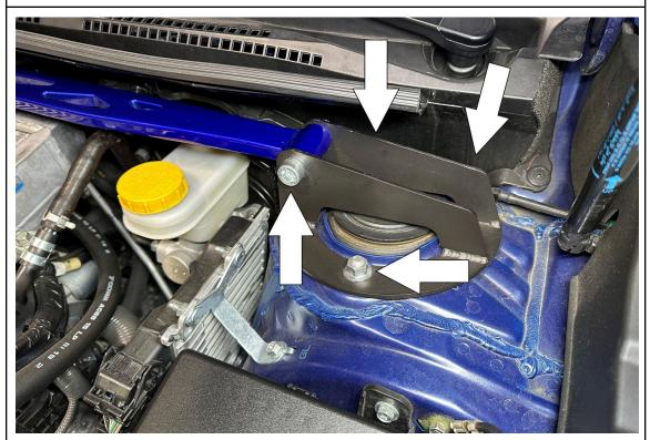
4. Loosely reinstall the original strut mount nuts. Loosely install the HPS strut bar using the two provided Allen head bolts and flange nuts.
