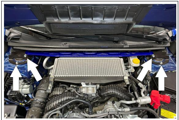
5. Once the strut bar is aligned and all fasteners are installed, fasten the six original strut tower nuts to 27 ft-lbs. Then, torque the Allen head bolts to 86 ft-lbs.
