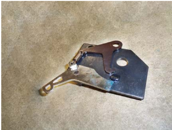
8. Remove reverse lockout assembly.
