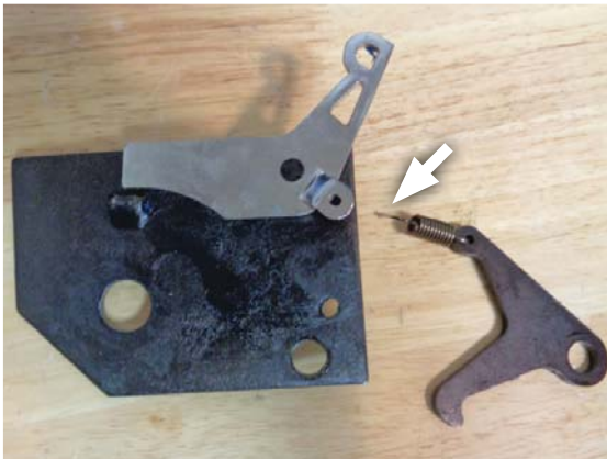
9. Disconnect detent arm spring from lockout arm.
