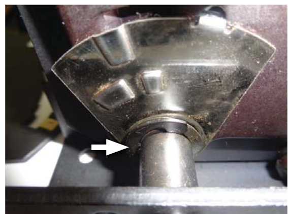
13. Secure assembly by installing e-clip (removed step 6) into groove on large pin.
