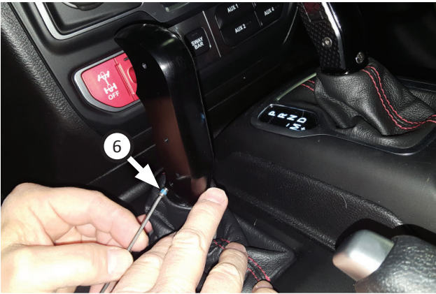
25. Remove SHS screws (x2) (3) and left shifter plate (2) from transfer case handle. Apply loktite to extended tip screw (6) then install into transfer case handle as shown.
