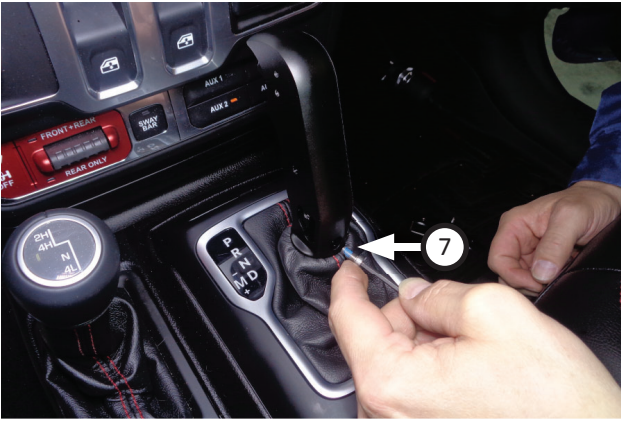
13. Apply loktite to SHCS screw (7) then install it into shift handle body as shown.
