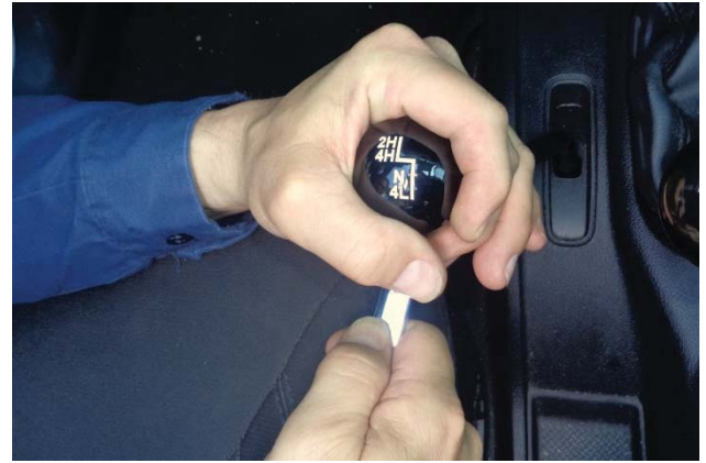
23. Tighten the jam nut against the knob.
