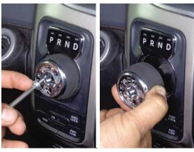
4. Remove screw from shifter knob then remove shifter knob from dial stem.
