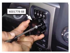
5. Set **shifter knob (4001778-88)** onto dial stem then fasten using screw (removed step 4).
