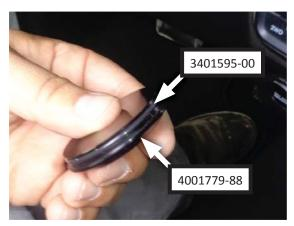
6. Fit **O-Ring (3401595-00)** into groove on **knob insert (4001779-88)**.
