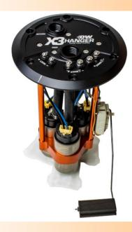
The new DeatschWerks X3 Ford F-150 Module is now available for the 1999-2004 model years, which includes accommodation for 1, 2 or 3 fuel pumps, and retention of ALL functionality of the OE module. The DW X-Series module consists of a billet top-hat, billet pump holder, and bracket for the OE fuel level sensor. These three components work together to deliver the flow you need and the OE functionality you want.
