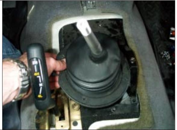
STEP 20. Reinstall rubber protective boot bolts.
