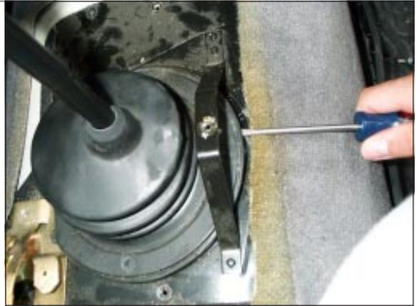
STEP 13. Remove bolts ① securing shifter to transmission.
