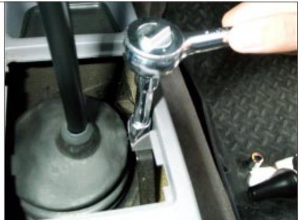
STEP 6. Remove center console bolt in cup holder.
