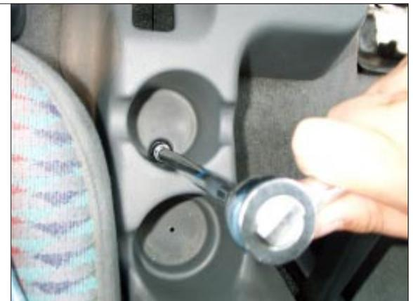
STEP 7. Remove center console bolts from storage console (a)
