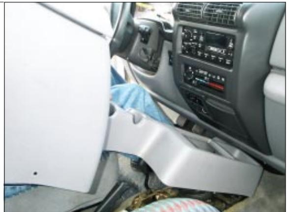
STEP 22. Install center console bolt near shifter.
