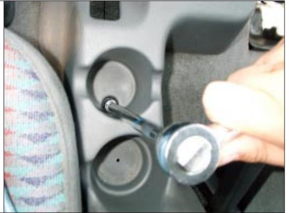
STEP 24. Install center console bolts from storage console (a)
