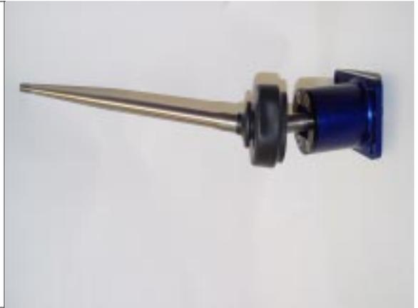
STEP 17. Either reuse stock gasket or apply RTV silicone sealant to shifter base.
