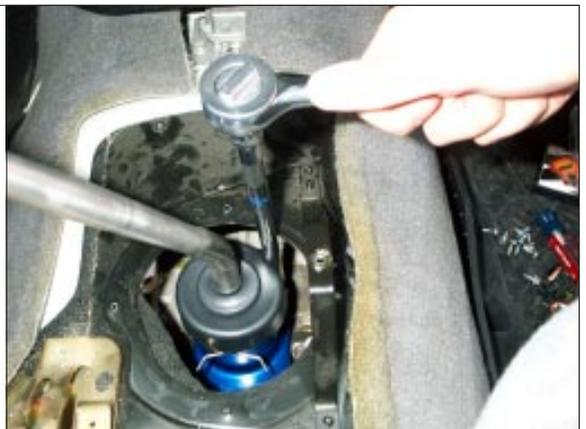
STEP 19. Reinstall rubber protective boot.
