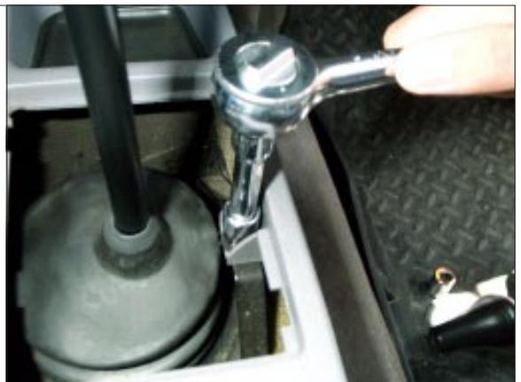
STEP 23. Install center console bolt in cup holder.
