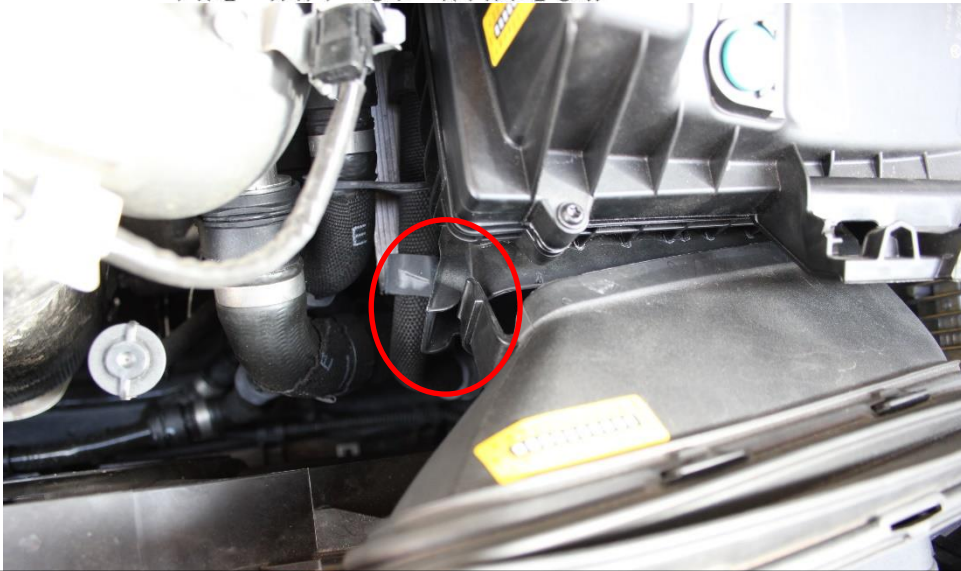
5. The plastic part of the duct can now be unclipped from the airbox and removed.
