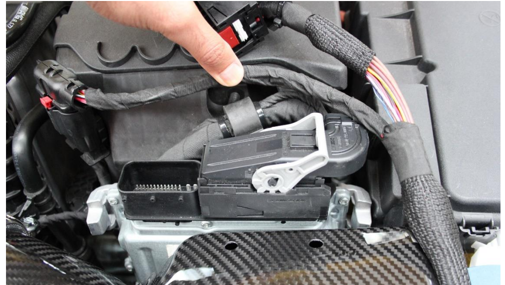
30. Reconnect the plugs starting with the one shown here. Make sure the clamps are pushed back down fully so that they lock.
