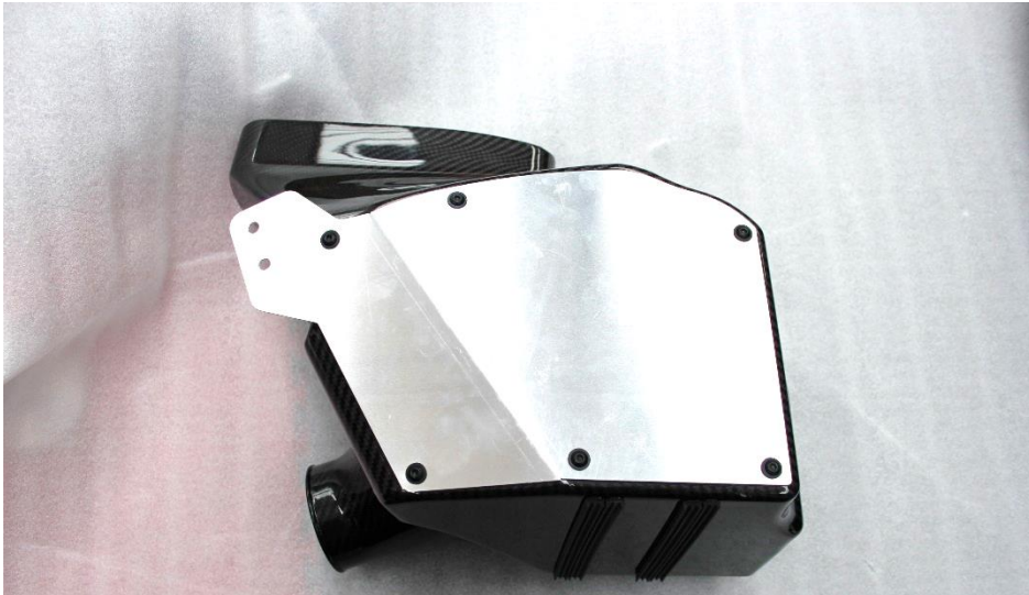
21. Secure the base panel onto the airbox with the supplied M5 screws. Photo shows a silver panel for contrast.
