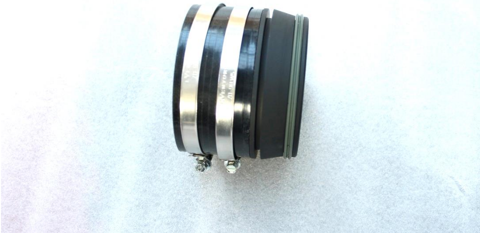
17. Push the supplied silicon coupler onto the flange with the hose clamps. Do not tighten the clamps yet.
