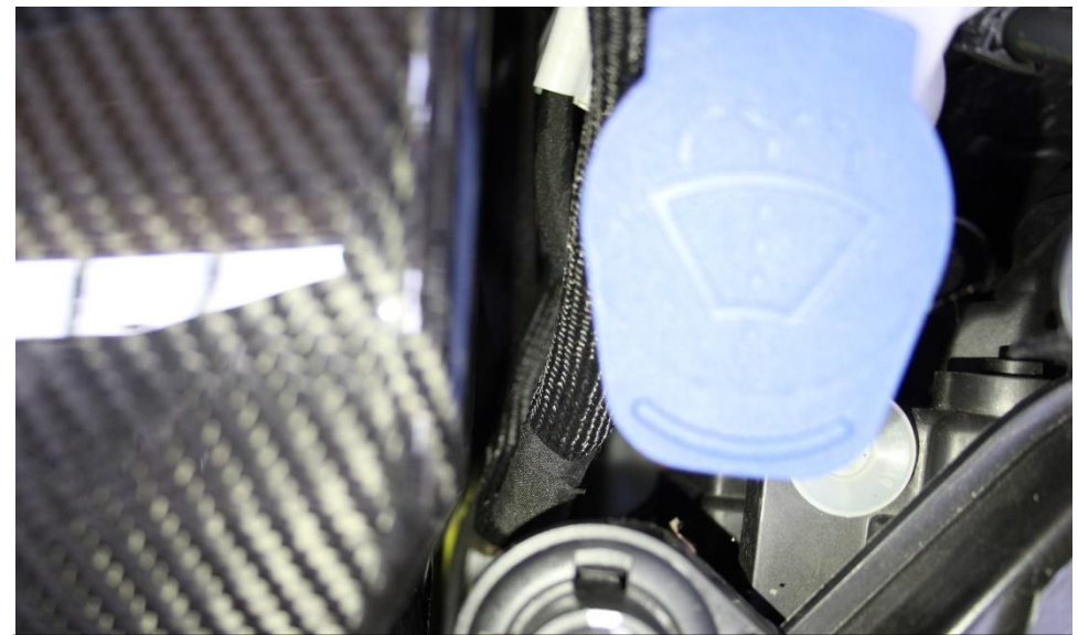
24. Make sure the loom on the right side is not trapped underneath the airbox.
