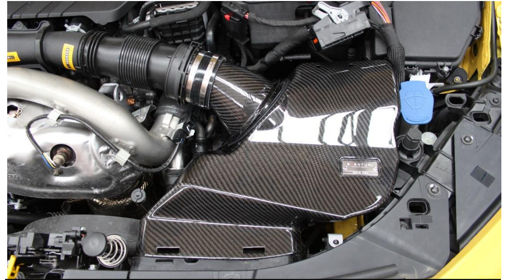
22. Lower the airbox into the engine bay and push the carbon tube into the silicon coupler.
