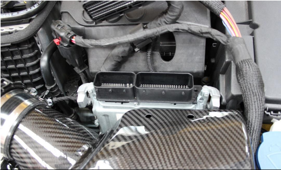
29. Carefully push the ECU down the back of the airbox so that it goes all the way down as shown.
