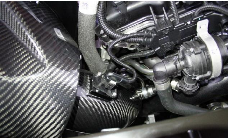
27. Connect the temperature sensor plug.
