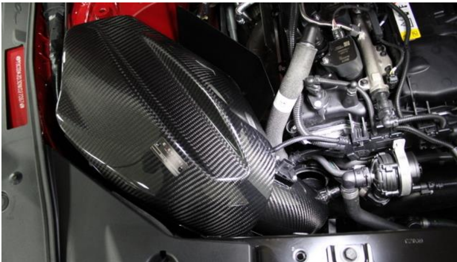
23. Lower the airbox with the tube angled downwards and ensure the mount and secondary scoop go into place as described previously.
