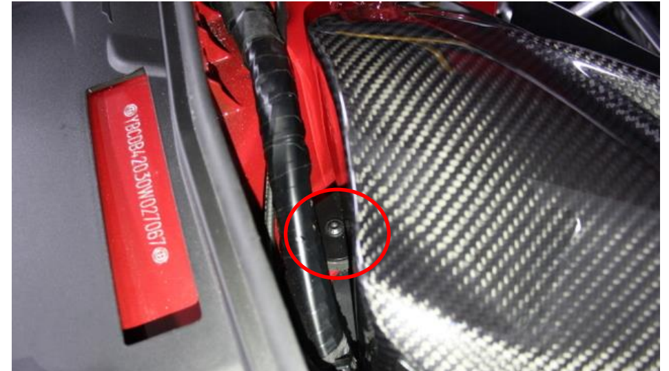
24. locate and push the top mount into the upper rubber bush.
