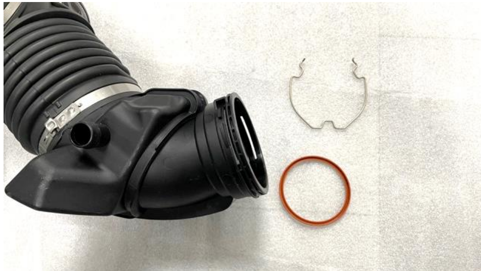
9. Remove the rubber O-ring from inside the OEM tube and also the spring clip.
