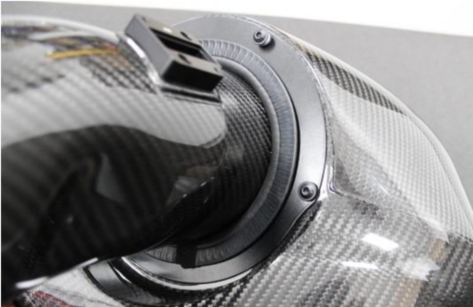
17. Another view of the sealing plate secured to the airbox.
