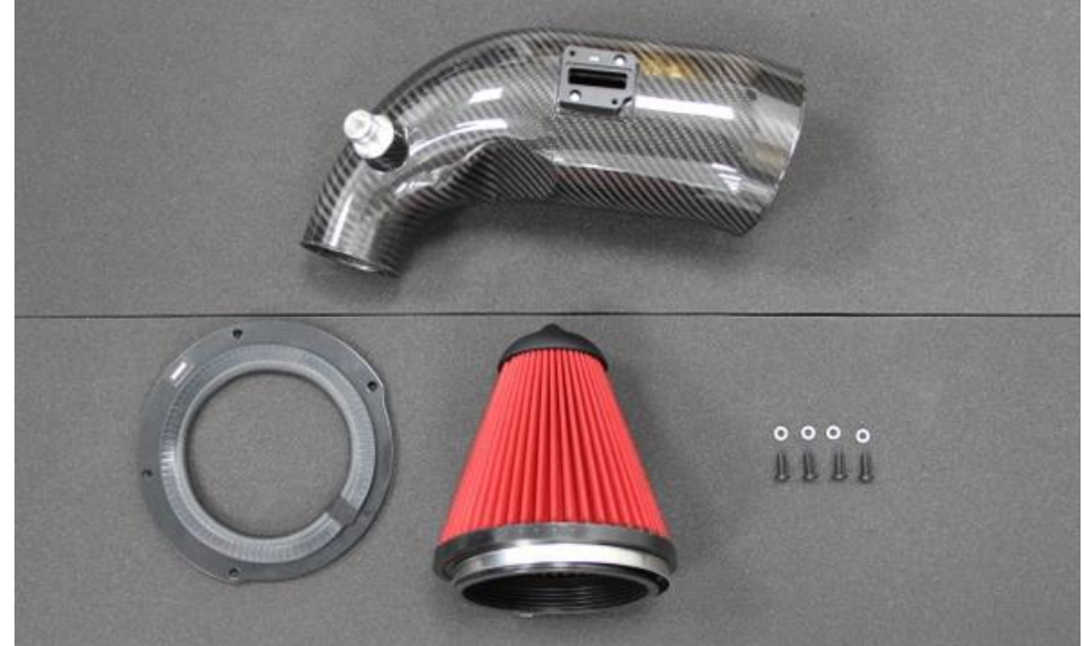
14. Take the inlet tube, filter, sealing plate and the M5 screws with lock washers.
