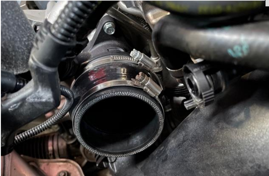
13. Install the flange assembly onto the turbo inlet – it will click into place.
