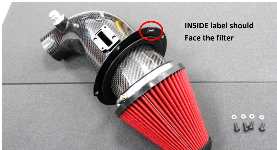
15. Push the sealing plate onto the tube – ensure the INSIDE label is facing the filter side. Now push the filter fully onto the tube and secure with the attached clamp.
