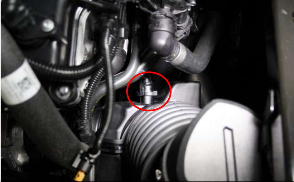
5. Remove the breather connector from the tube.
