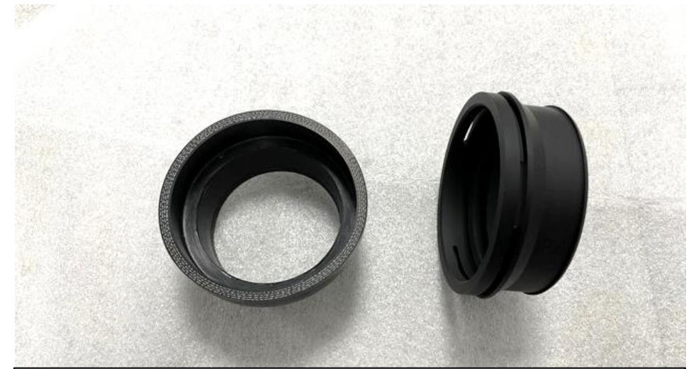
8. Take the machined flange and the silicon reducer – we will now prepare these for installation onto the turbo inlet.
