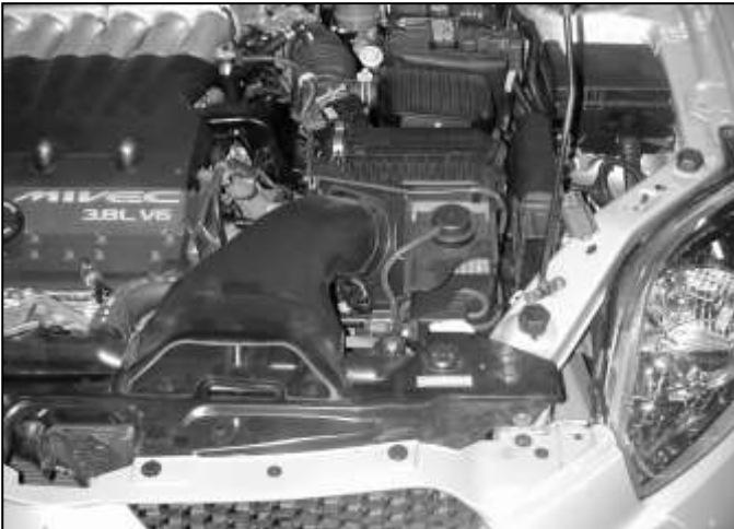
a. Factory airbox system installed.
