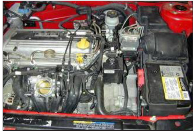
f. Release the inlet tube from the throttle body and air box, then remove the inlet tube from the engine bay.
