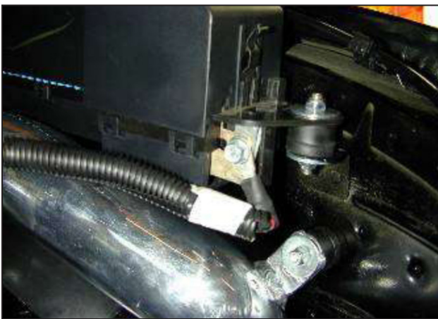
n. Secure the fuse block to the rubber mount with a lock nut and washer. Confirm that all wires are routed correctly.
