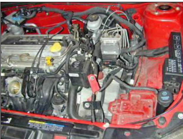
i. Remove the air box from the vehicle.
