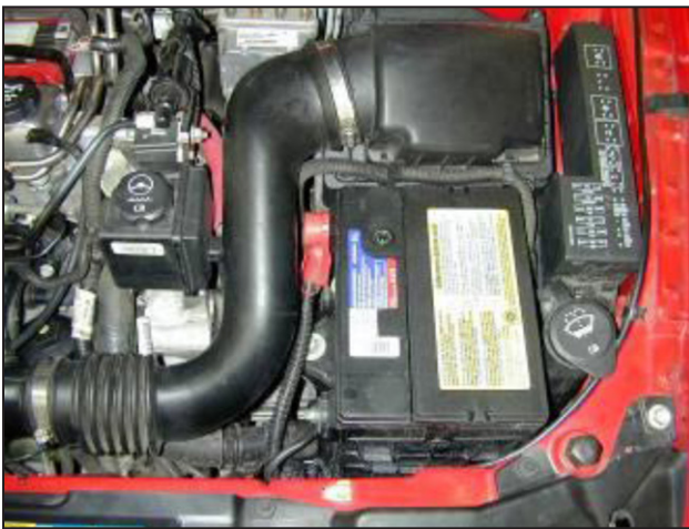
a. Stock air box system installed.
