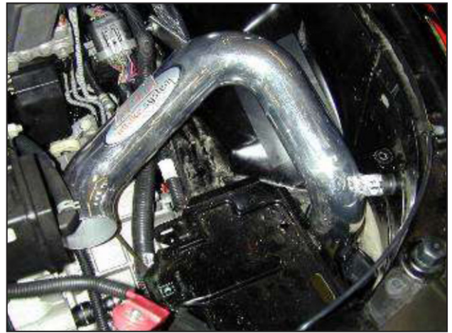
g. Place the intake pipe in engine bay as shown. Do not tighten any bolts or nuts.
